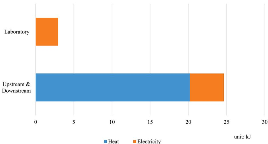
Fig. 5. Energy requirement for synthesizing one 3 cm by 3 cm organic battery cell.
