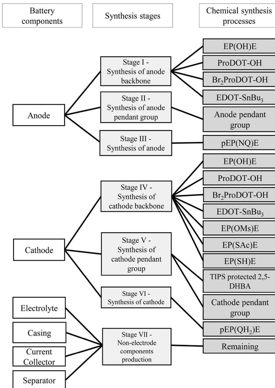
Fig. 3. The chemical synthesis processes are categorized in seven synthesis stages for the assembly of the six components of the all-organic battery cell.
