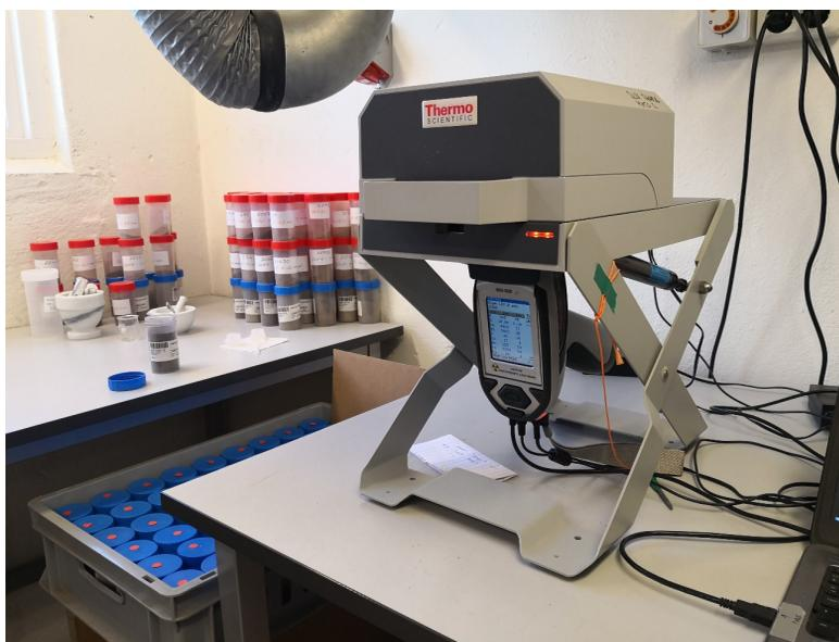
Figure 4: Image of the portable X-ray fluorescence (PXRF) device used, shown mounted on its purpose-built frame with the lid closed.
