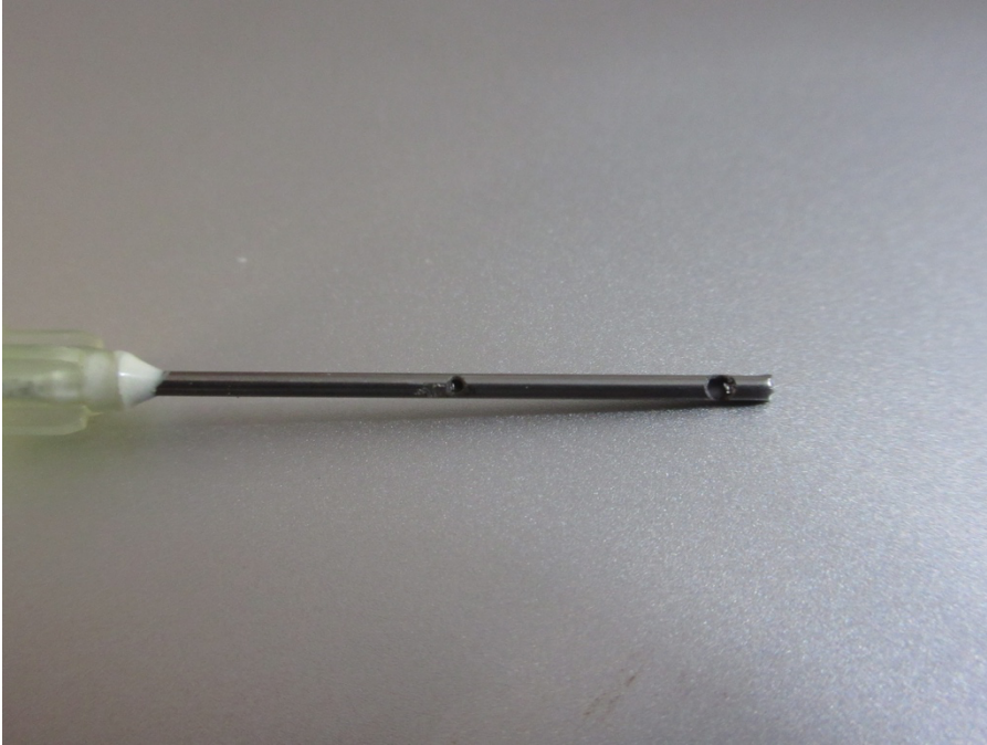
Figure 2 Hypodermic needle for heated probe.
