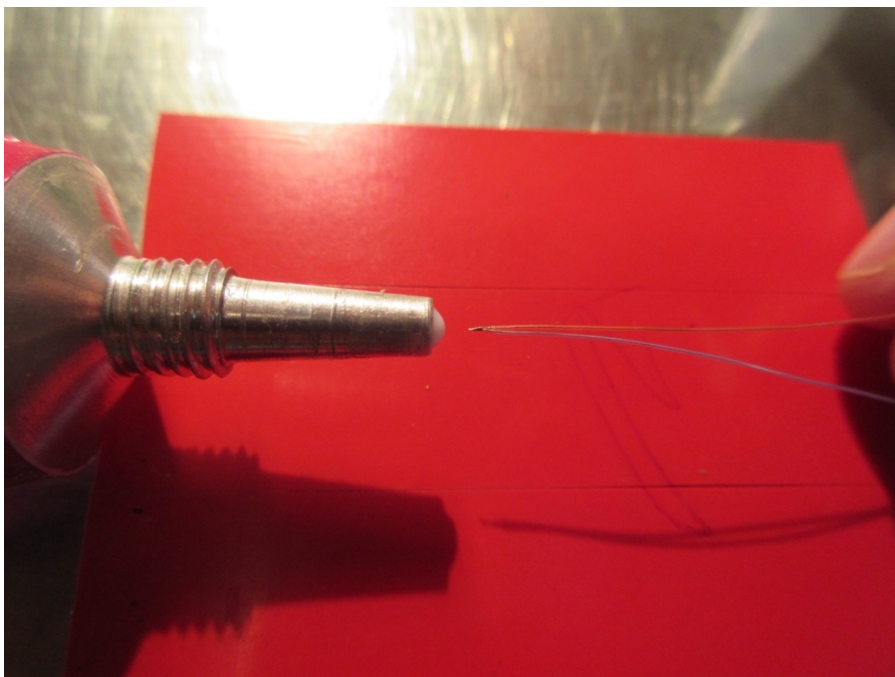
Figure 5 Inserting thermocouple in acrylic glue for electric isolation
