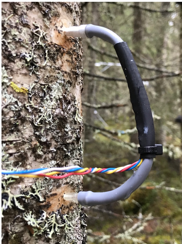
Heat dissipation sensor, installed in a Betula pendula tree
