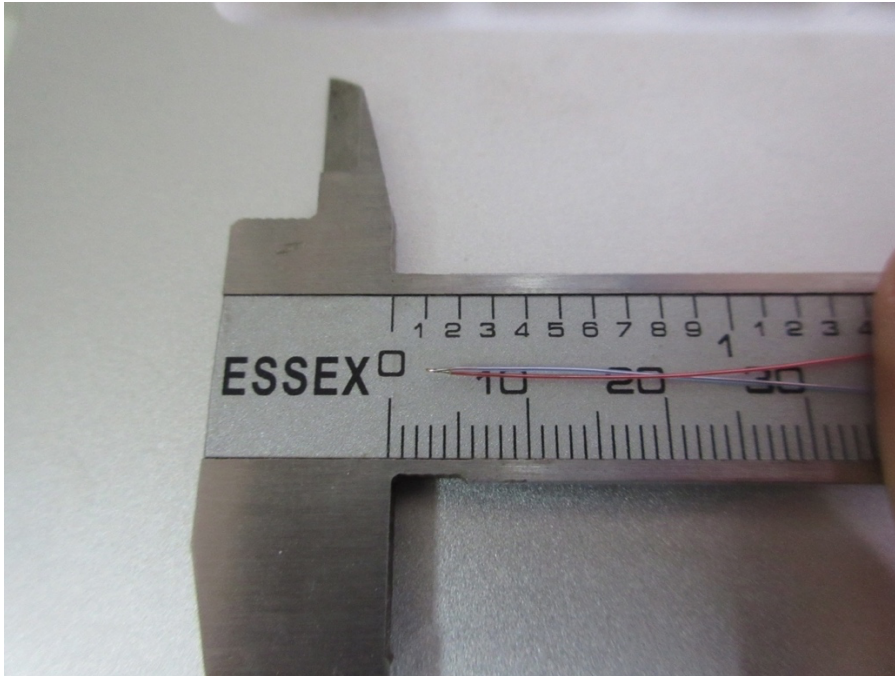
Figure 4 Type-T thermocouple with constantan and insulated copper wire
