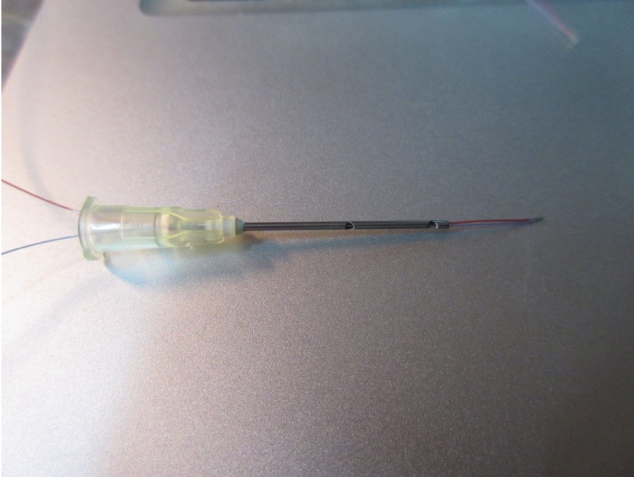
Figure 6 Hypodermic needle with thermocouple during initial assemblage
