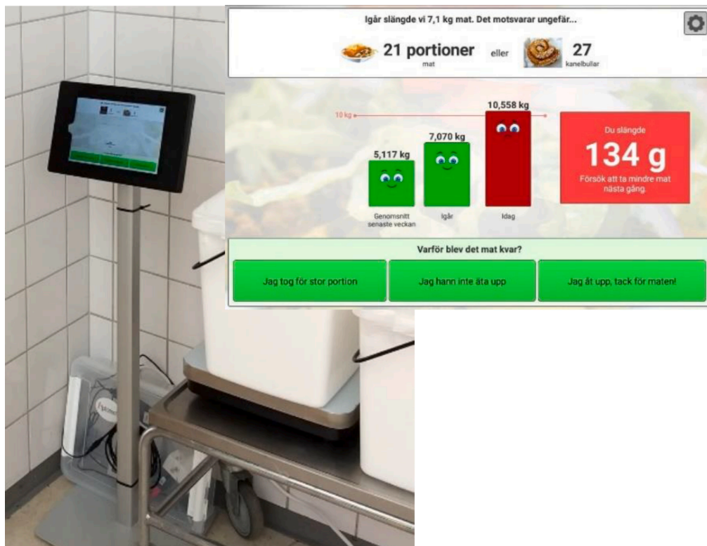
Fig. 4. Plate waste tracker at the point where school canteen guests scrape their plates. The interface communicates the target that the canteen has set and also shows how much plate waste was generated previously. The impact of the waste is shown in indicators that guests can relate to, such as “Yesterday we threw away 7.1 kg, which is roughly the same as 21 portions or 27 cinnamon buns”. The interface also allows guests to give feedback on why they wasted food.
