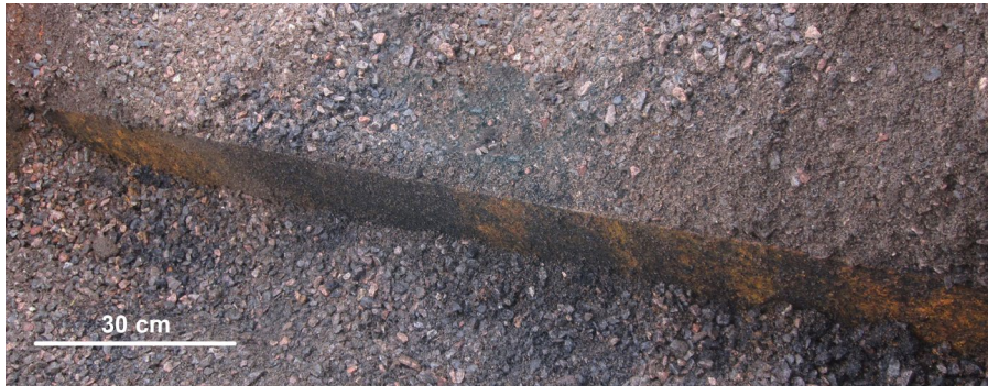
Figure 9. Iron oxide deposits on a sheet metal inner dividing wall in the bioreactor in paper I. The photo has been modified in Photoshop. A glove positioned in the upper part of the picture, indicating size, has been replaced by gravel.
