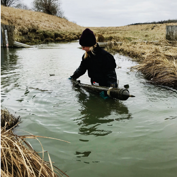
Figure 4. Collection of fluvial suspended sediment from a Phillips sampler in catchment C6. Photo by Mikael Östlund.
