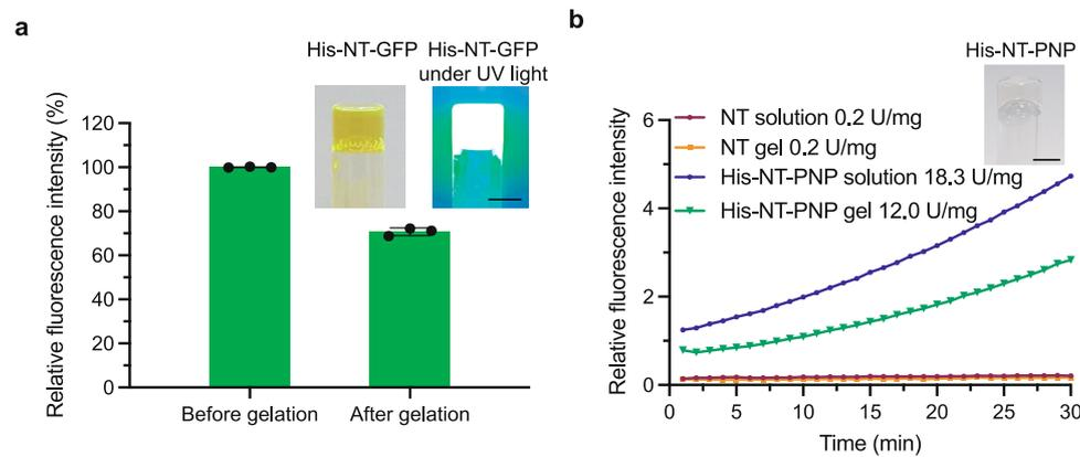
**Fig. 6 | NT fusion proteins form hydrogels with intact activity of the fusion partner. a** Relative fluorescence intensity before and after gelation of His-NT-GFP (300 mg/ml) and inverted vials containing His-NT-GFP hydrogels (300 mg/ml) under visible and UV light. Dots show individual measurements ( $n = 3$ ) and error bars show standard deviation. Center of the error bar shows the mean.
