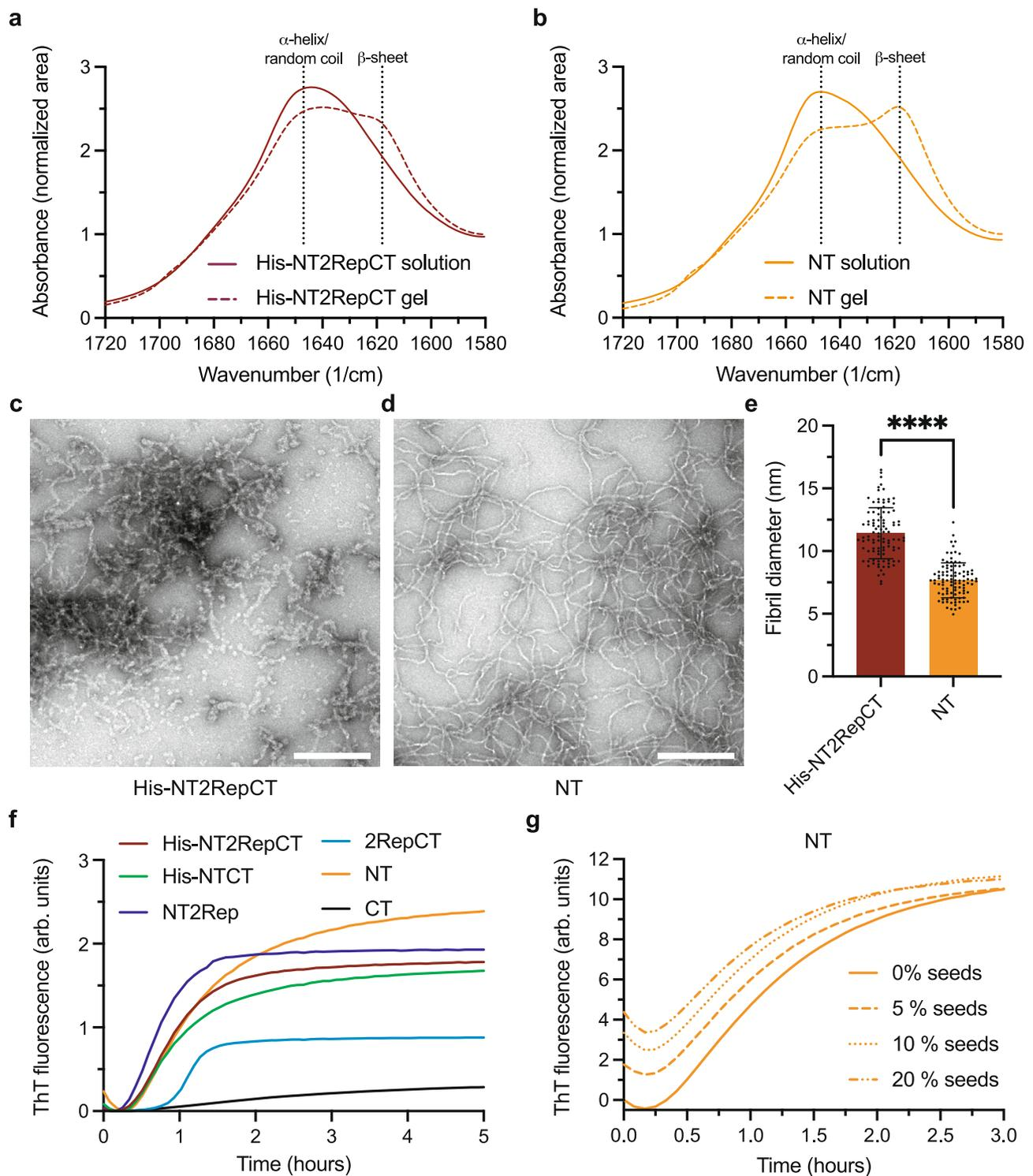
**Fig. 3 | Structural changes during hydrogel formation.** **a** FTIR absorption spectra of His-NT2RepCT and **b** NT (both at 500 mg/ml) before (solution) and after (gel) incubation at 37 °C. **c** TEM image of a resuspended 50 mg/ml NT2RepCT and **d** NT gel. Scale bars are 200 nm. **e** Fibril diameters of His-NT2RepCT and NT hydrogels.  $n = 100$  fibrils measured,  $p < 0.0001$ . Error bars show standard deviation. Center of
