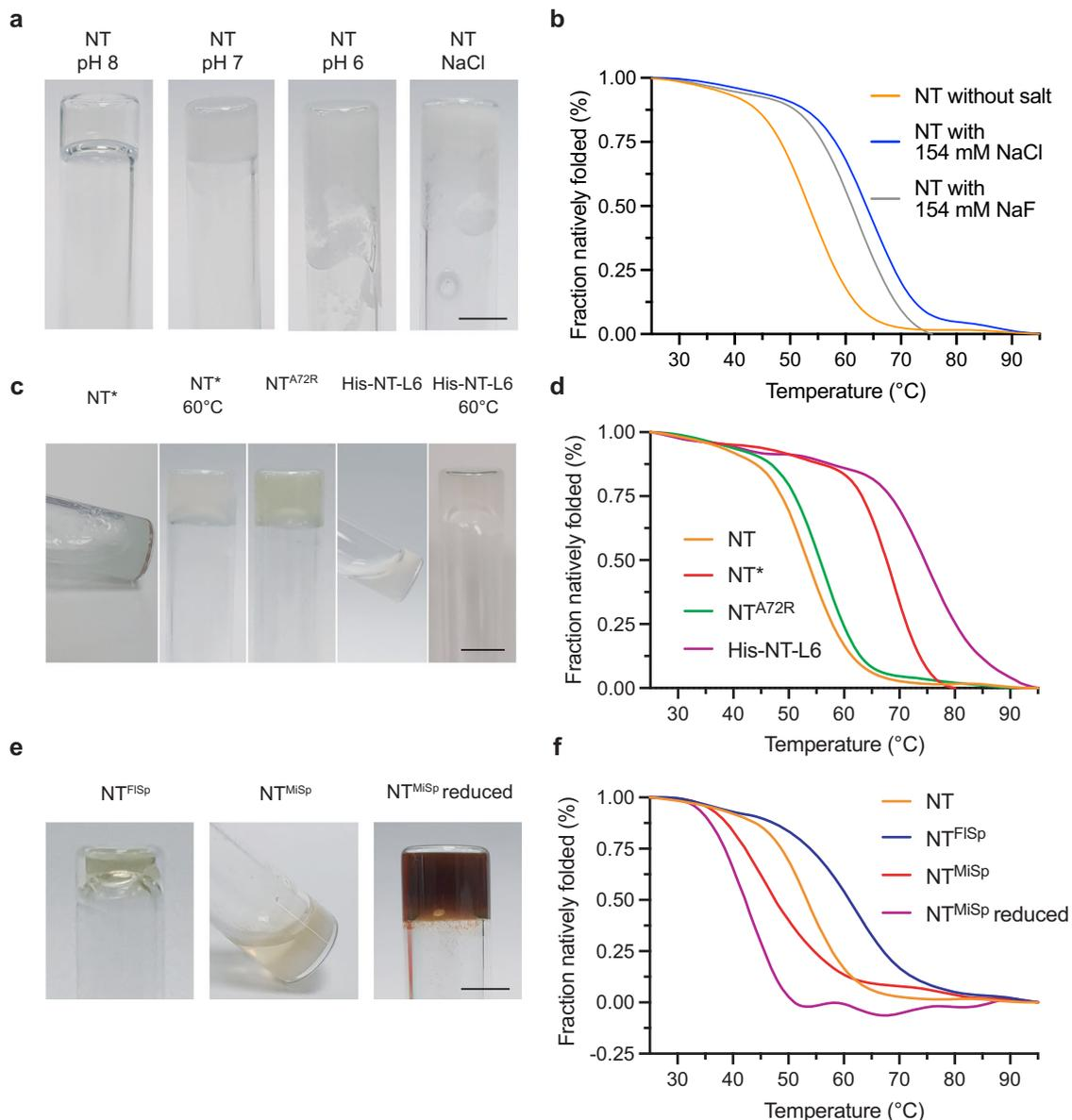
**Fig. 5 | Hydrogel formation of different NTs and their thermal stability.** **a** Vial inversion tests of NT (100 mg/ml) at pH 8, 7, 6 and with 154 mM NaCl (pH 8) after incubation at 37 °C. **b** CD spectroscopy of NT with and without 154 mM NaF and 154 mM NaCl, respectively. Molar ellipticity at 222 nm converted to fraction natively folded. **c** Vial inversion test of NT mutants (100 mg/ml) NT\* (37 °C and 60 °C) NT<sup>A72R</sup> (37 °C) and His-NT-L6 (37 °C and 60 °C). **d** CD
