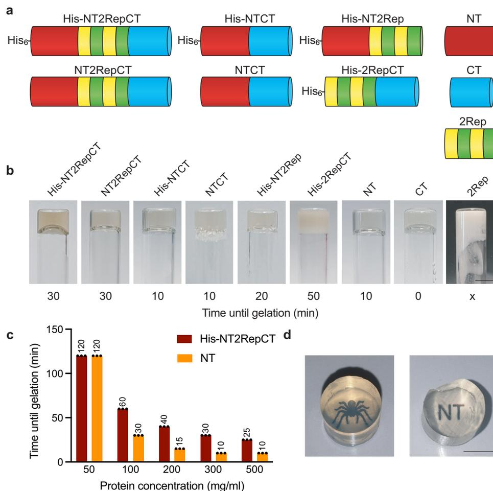
**Fig. 1 | Temperature-induced hydrogel formation of His-NT2RepCT and its different domains.** **a** Schematic presentation of the different spidroin constructs investigated herein. **b** Gelation times of the different recombinant spidroins (300 mg/ml) at 37 °C as tested by vial inversion. CT gelled immediately without incubation (<300 mg/ml) and 2Rep precipitated (300 mg/ml, scale bar is 5 mm).
