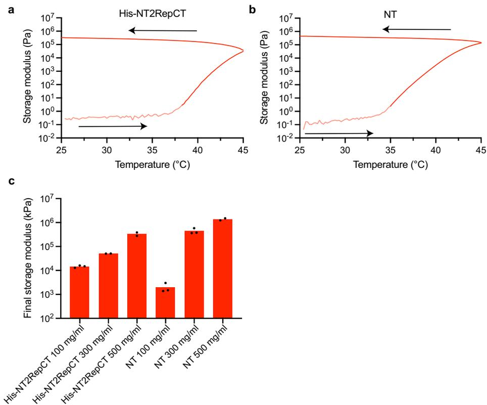
**Fig. 2 | Rheological analyses of His-NT2RepCT and NT gelation.** **a** Temperature ramp during oscillatory measurement of His-NT2RepCT (300 mg/ml) and **b** NT (300 mg/ml). Arrows indicate temperature course, lighter shaded portions of the storage modulus data depict testing below the manufacturers stated lower torque
