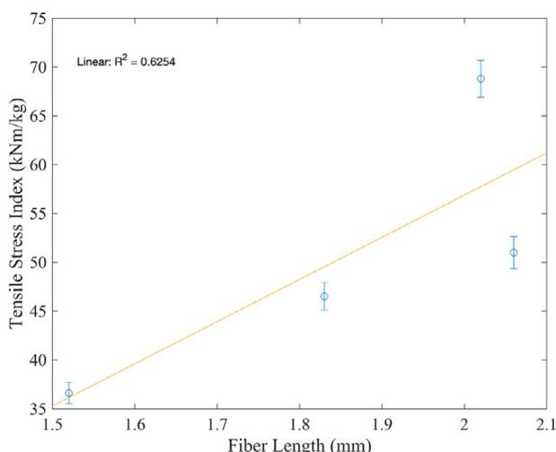
**Figure 7:** Tensile stress index plotted against fiber length with a linear regression to indicate the trend.
