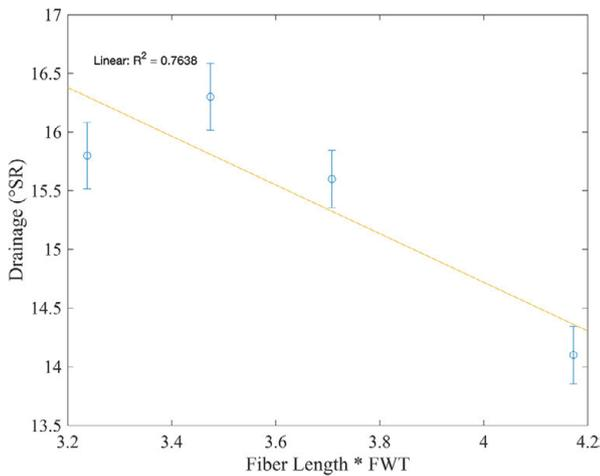
Figure 6: The product of fiber length and Fiber wall thickness plotted against drainage with a linear regression to indicate the trend.
