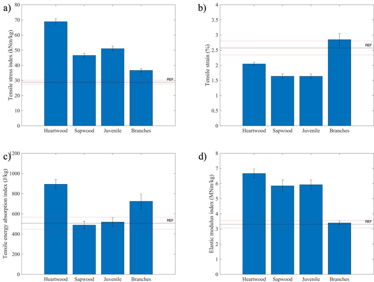
**Figure 4:** (a) Tensile strength index (kNm/kg), (b) Elongation at break (%), (c) Tensile energy absorption (J/kg), and (d) Elastic modulus index (MNm/kg) for sheets made of the pulps, the error bars indicate a 95 % confidence interval based on ten measurements. Reference pulp mean value is shown with a solid black line with dashed red lines representing 95 % confidence interval.
