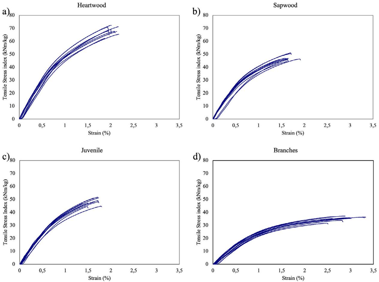
Figure 5: Stress-strain curves for Heartwood (a), Sapwood (b), Juvenile wood (c) and Branches (d).
