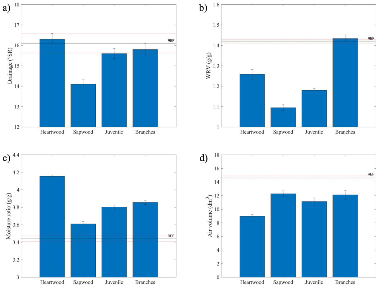
**Figure 3:** (a) Drainage (°SR), (b) Water retention values (g/g), (c) Moisture ratio (g/g) after 20 ms vacuum dewatering at  $-40$  kPa, and (d) Penetrated air volume (dm<sup>3</sup>) during 20 ms vacuum dewatering at  $-40$  kPa, for all pulps, the error bars indicate a 95 % confidence interval based on four measurements. Reference pulp mean value is shown with a solid black line with dashed red lines representing 95 % confidence interval.
