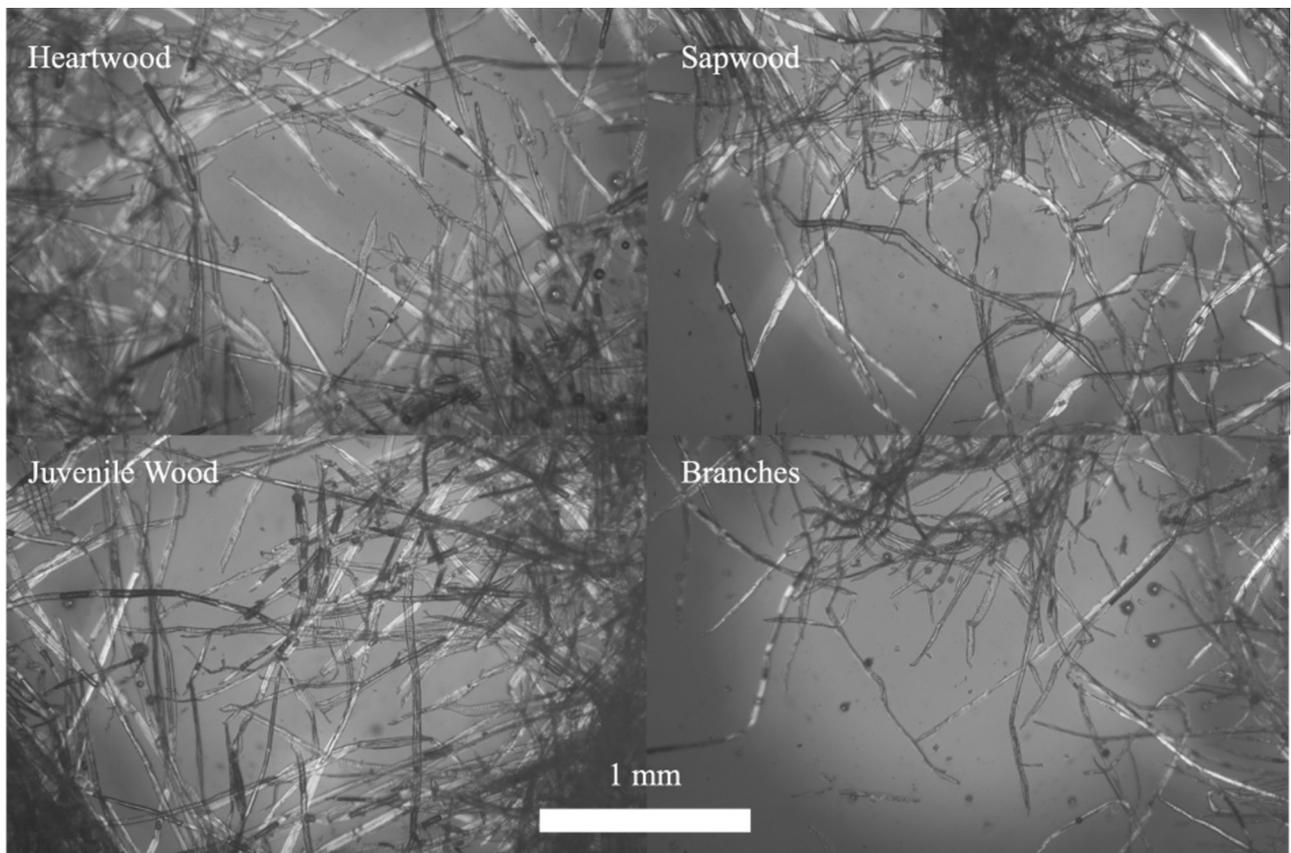
**Figure 2:** Optical microscopy images of the four pulp types. All four images have the same magnification and the scale is indicated by the white bar of 1 mm.
