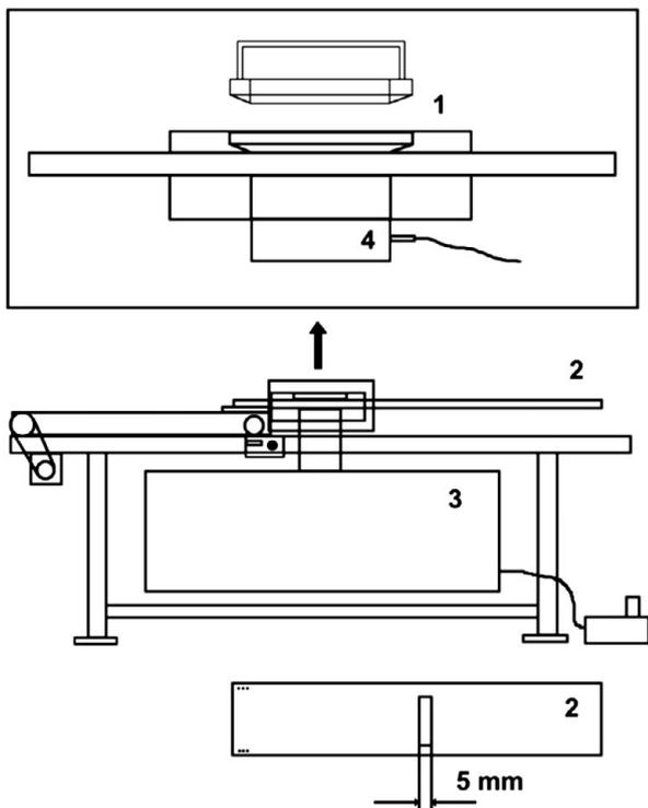
**Figure 1:** Schematic picture of the laboratory suction box. The machine includes: (1) sample frame, (2) moveable plate with 5 mm rectangular opening, (3) 300 L vacuum tank, and (4) a transducer logging the pressure directly underneath the sample. Redrawn from Granevald et al. (2004).
