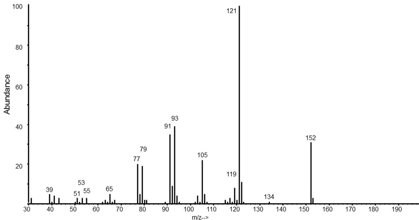
FIGURE 3 EI mass spectrum of unknown A, identified as *p*-mentha-1,3-dien-9-ol
