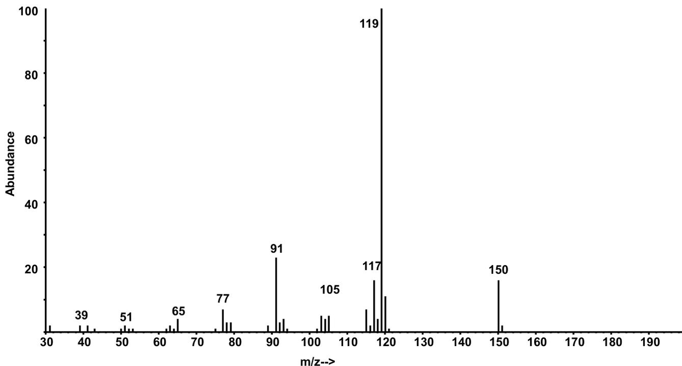
FIGURE 2 EI mass spectrum of unknown B, identified as *p*-cymen-9-ol
