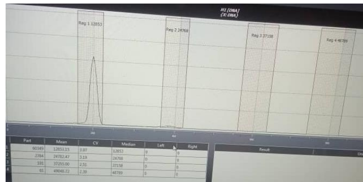
Figure 5.12. A peak curve at channel 200 in region one indicates a well-calibrated machine.
