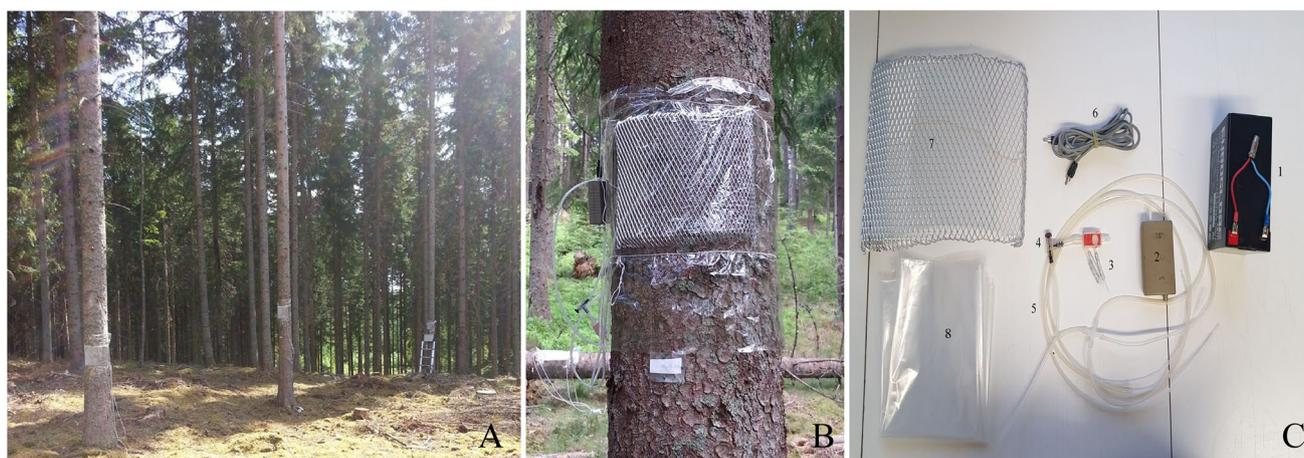
**Fig. 1** Setup used for headspace collections from logs of Norway spruce trees (*Picea abies*) through the different stages of *Ips typographus* attack. **A**) three sampled standing trees in one of the field sites; **B**) metal grid covered with a polyester roasting bag that was wrapped around the tree bark forming an enclosure for odor collections; **C**)
