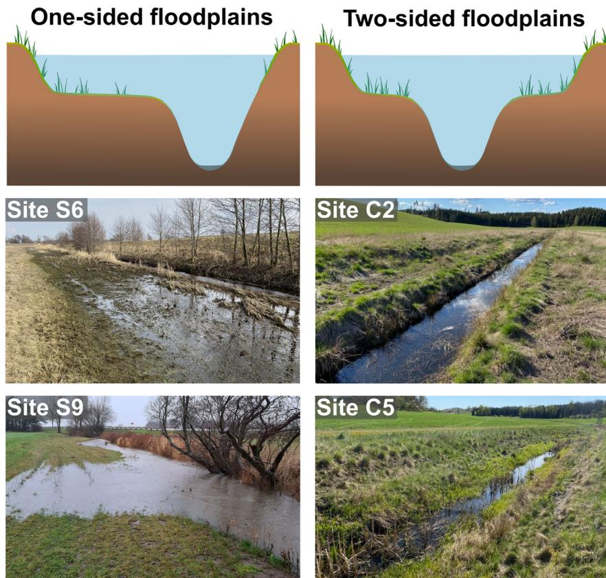
Figure 2. Cross-section profiles of floodplain remediation with one-sided and two-sided floodplain designs. Four floodplain remediated streams included in papers I-III with one-sided floodplains (sites S6 and S9) and two-sided floodplains (sites C2 and C5). Photographs by Lukas Hallberg. Adapted from paper III.
