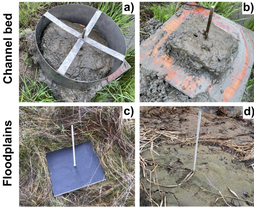
Figure 5. Plates for collection of deposited sediments installed on **a-b)** channel beds and **c-d)** floodplains. **a)** Cylindrical frame used for collecting channel sediments. **b)** Sampled plate area. Photos by Lukas Hallberg.
