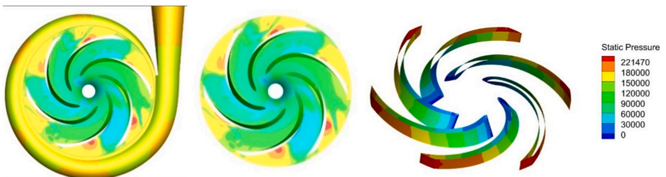
Fig. 9. The figure depicts the static pressure distribution contour over the pump impeller and volute.
