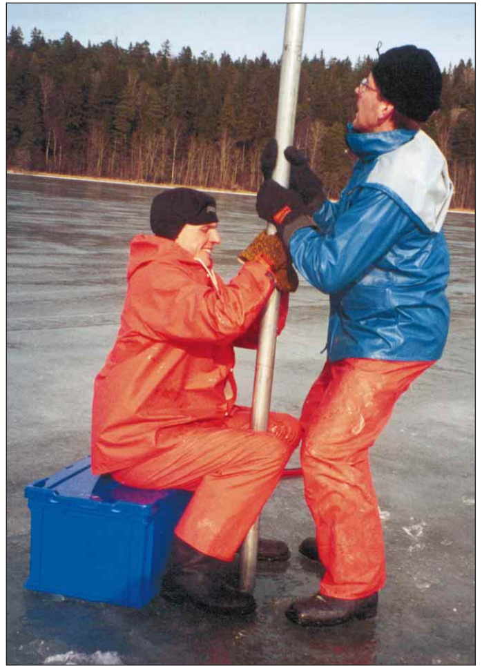
The master core from Södra Björkfjärden was taken in summer, while the additional long cores from Gisselfjärden and Asköfjärden and from the small forest lake Fågelsjön were collected in winter using a freeze corer (left) and a Russian peat corer operated with rods (right). The freeze corer, shown here, just before lowering it into the lake sediment, allows the taking of undisturbed cores of unconsolidated surface sediments. The freeze corer is filled with dry ice and the sediment freezes in situ in the lake bottom. Photo: C. Savage.
