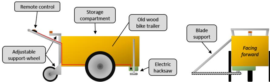
Figure 2. Schematic illustration of an in-house built harvester used to cut herbage at different locations.
