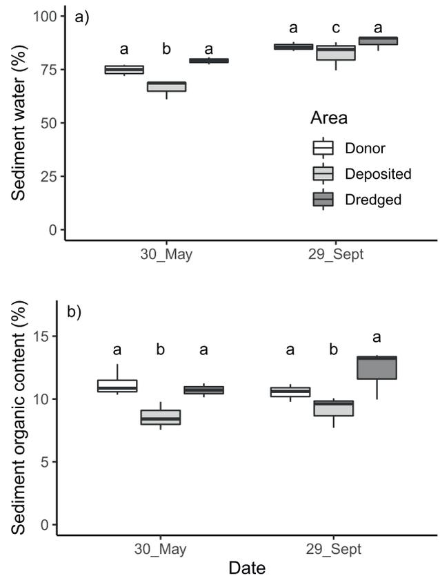
Fig. 6. Sediment water content (a) and organic content (b) in the donor area (undisturbed sediment), the dredged area and the transplant area (deposited sediment),  $N = 4$  for each area on each date. Significant differences ( $p < 0.05$ ) between areas and over time are indicated with lowercase letters.
