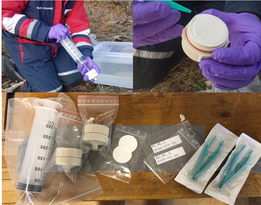
Figure 1. Equipment used for eDNA sampling consisting of plastic syringe, Swinnex filter holder, membrane filters (CN and GMF), zip-lock bags and forceps. Photo: Göran Sundblad/Erik Karlsson ( Paper II ).
