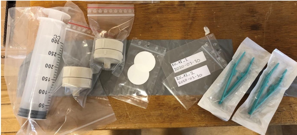
Figure S1. Sterilized equipment ready to be used for mesocosm sampling 2020 (left to right); 300ml syringe, Swinnex filter holders pre-loaded with filters, extra filters, sample bags, plastic forceps.
