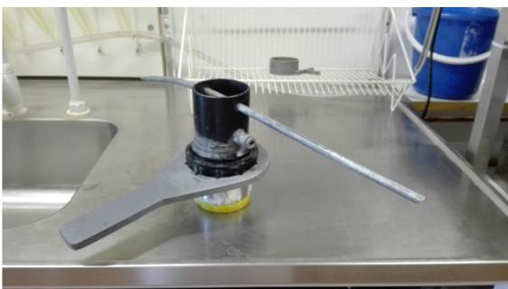
*Figure 31. Black top cylinder screwed in place onto the black base cap and tightened.*
