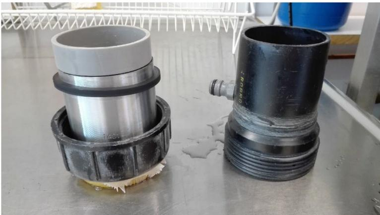
*Figure 33. Soil cylinder sample (10 cm cylinder) with parts to be joined.*
