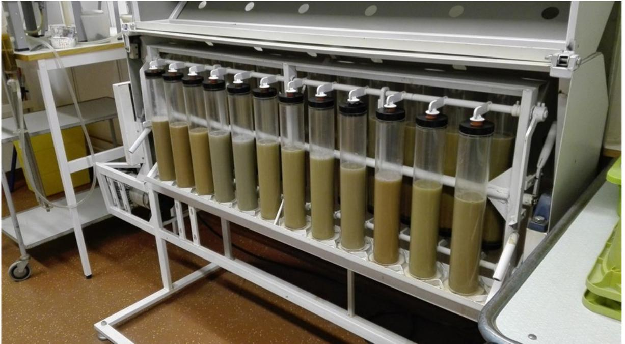
*Figure 3. Samples in the rotator ready for shaking overnight.*
