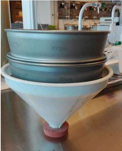
Figure 6. Sieves on top of the funnel for wet-sieving.
