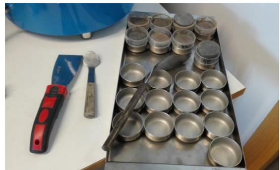
*Figure 25 (left). Removing samples from rings.
