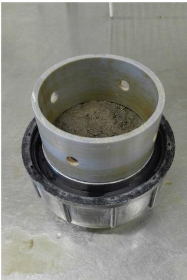
*Figure 30. Set-up (5 cm soil samples) with black base cap (threaded sleeve to attach soil sample to the water head control black top cylinder, see Figure 29), rubber ring (seal) and upper grey ring (to concentrate water flow onto the soil sample surface).*
