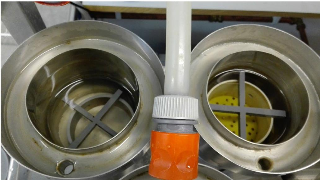
*Figure 28. Container for measuring saturated hydraulic conductivity using (left) 10 cm high cylinders and (right) 5 cm high cylinders, as regulated with the height adjustment equipment at the base.*
