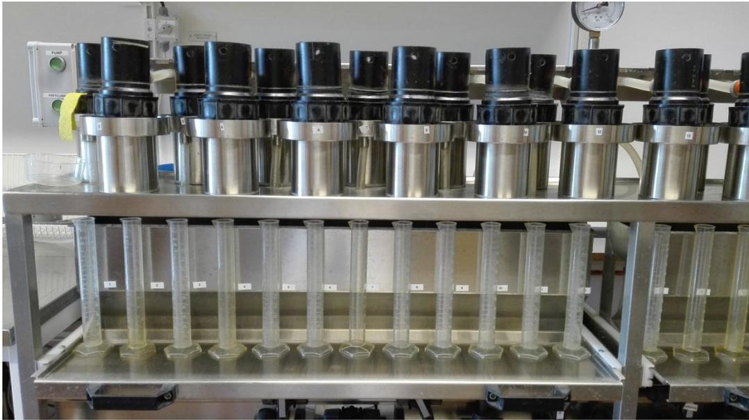
*Figure 47. Samples placed in the permeameter ready for starting the measurements.*
