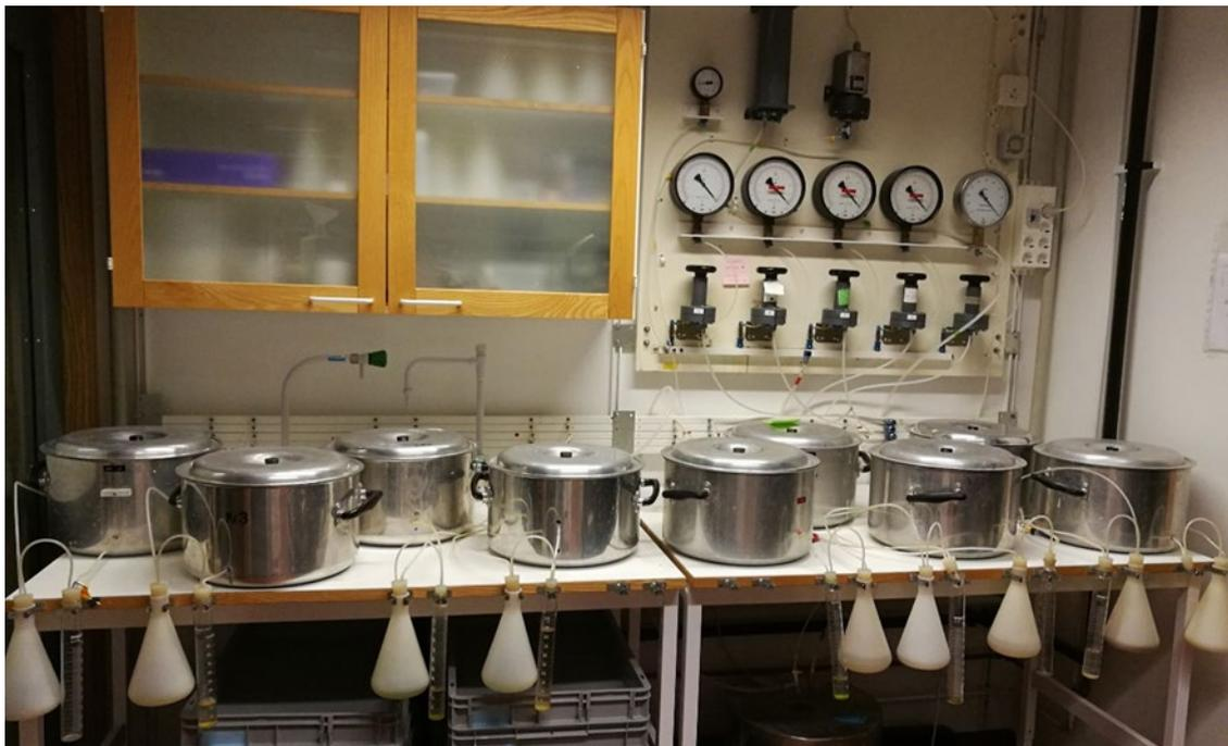
*Figure 11. Pots with ceramic porous plates connected to the laboratory vacuum system.*
