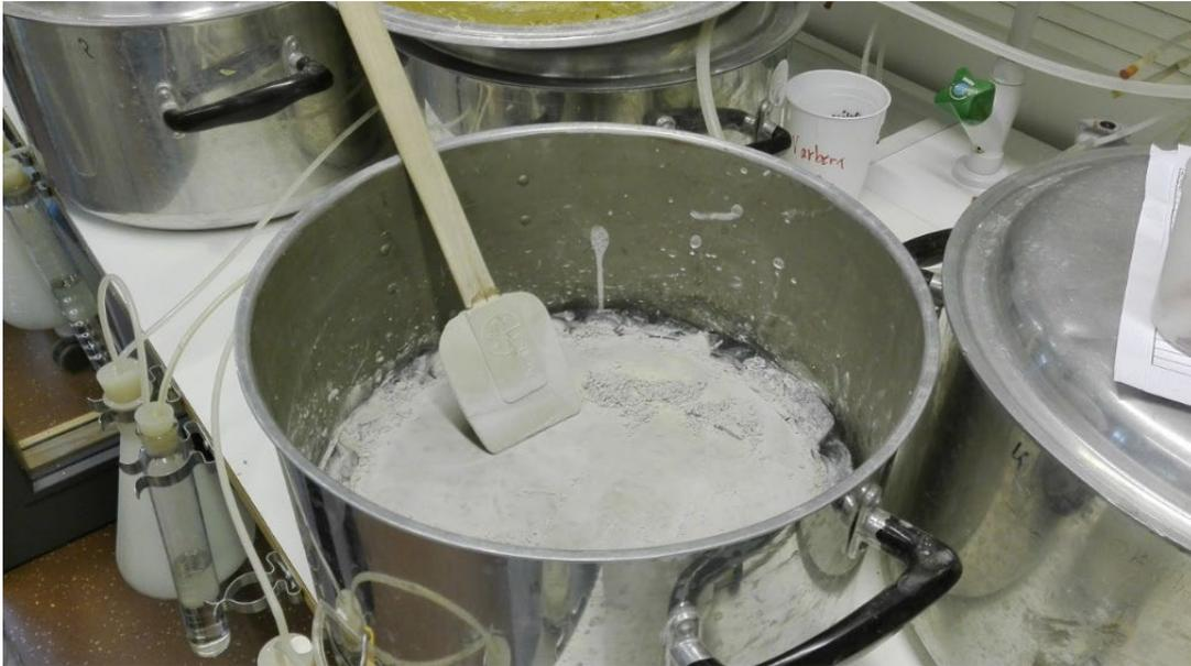
*Figure 17. Pot and (inside) plate covered with white quartz powder slurry.*
