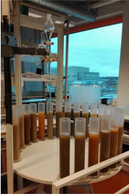
*Figure 5. Samples on the table ready to start the pipette method experimental run.*
