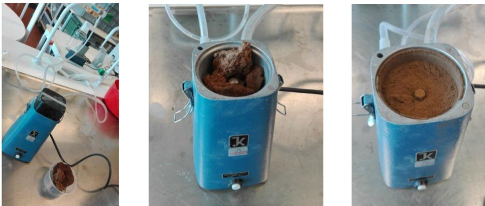
Figure 9. Specialist mill used for crushing peat soil samples containing hard charcoal-like concretions.
