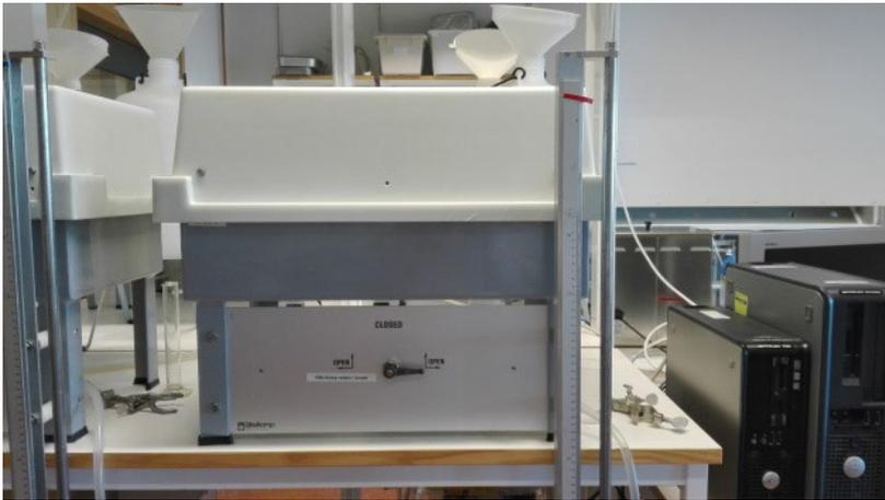
*Figure 10. Sandbox (model 08.01, Eijkelkamp) used to apply relatively small suctions to soil samples (from near zero to 1 m).*
