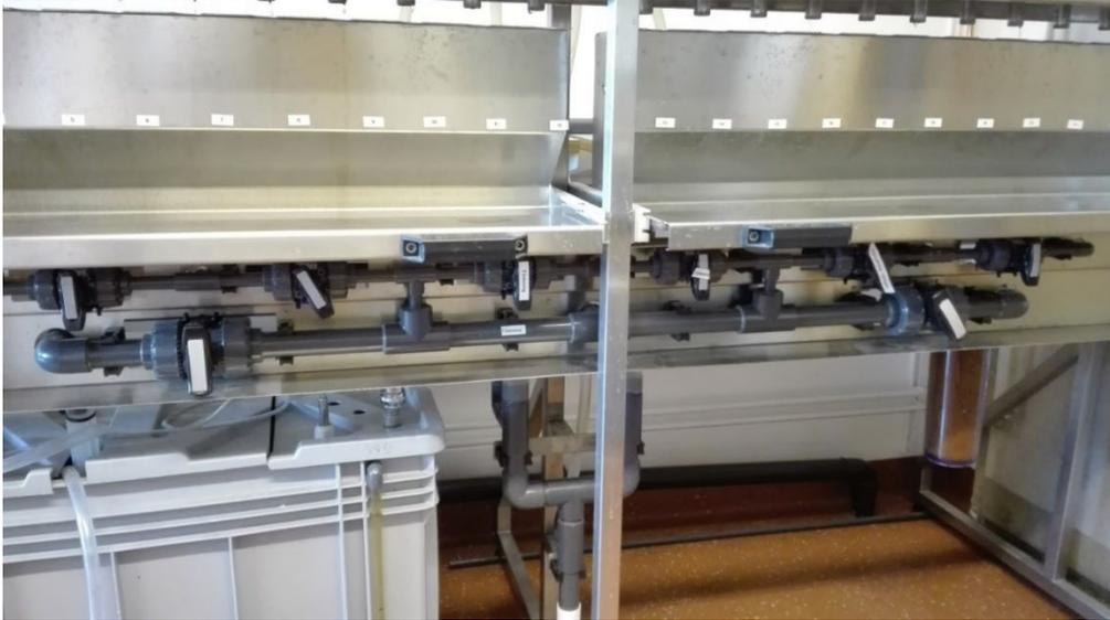
*Figure 48. Permeameter valves and water tank.*
