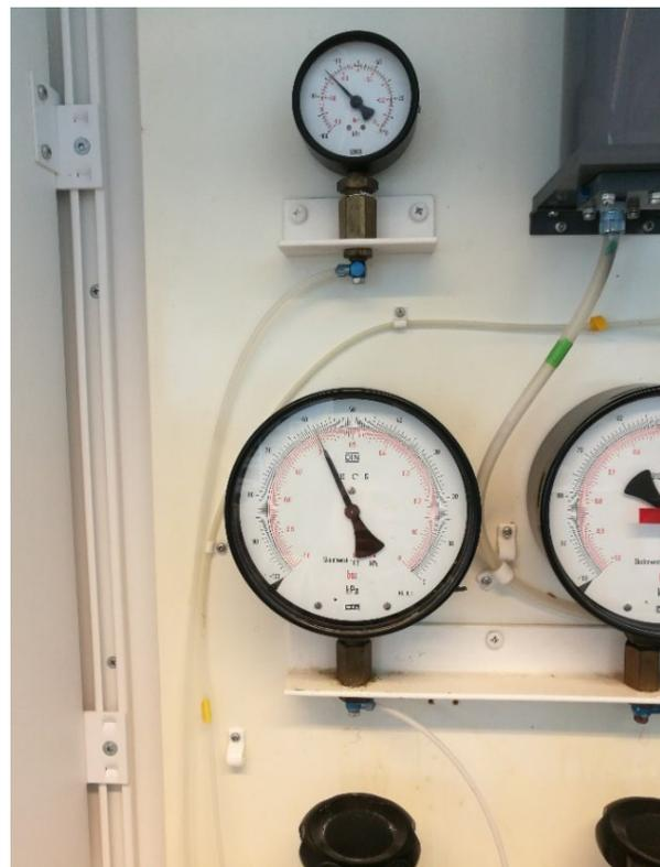
*Figure 14 (right). General pressure regulator for establishing the desired suction (on top).*
