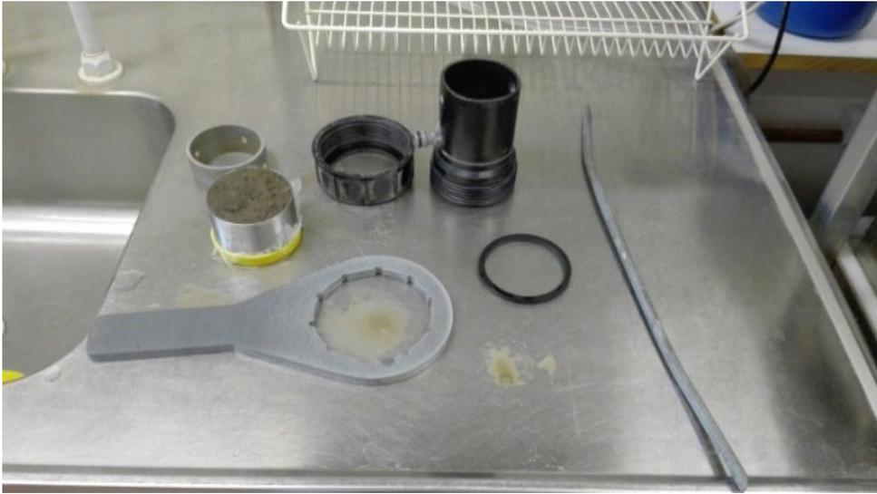
*Figure 29. Soil cylinder sample (5 cm height) and attachments to be joined.*
