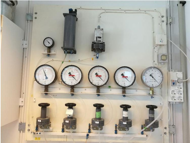
*Figure 12. Valves used to adjust suction to the desired setting.*
