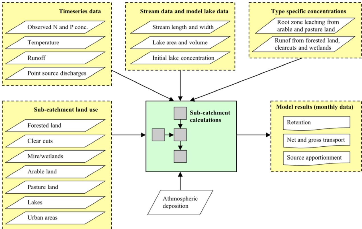
Figure 1. The structure and characteristics of inputs and outputs of the model.
