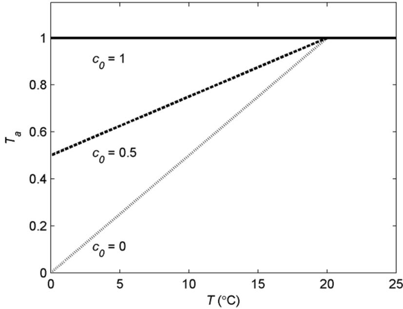
Figure 3. The influence of  $c_0$  on the temperature dependence of  $T_a$ .
