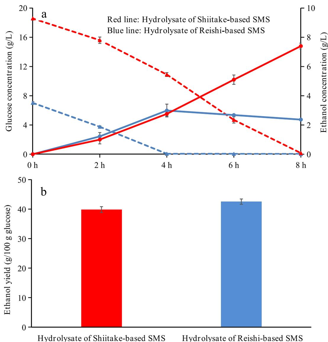
**Fig. 6.** Glucose consumption (dotted line) and ethanol production (solid line) (a) during *S. cerevisiae* fermentation of hydrolysates of shiitake-based SMS (red) and reishi-based SMS (blue) (10 % wheat straw addition). Ethanol yield (b) of SMS hydrolysates. Data refer to mean values  $\pm$  standard error (SE).
