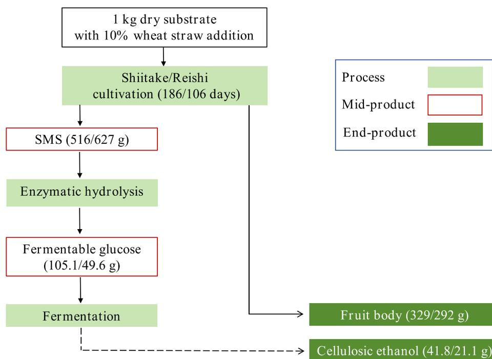
**Fig. 7.** Schematic of the concept and mass balance for the combined production of shiitake and reishi mushrooms and cellulosic ethanol from a substrate with 10% wheat straw addition.
