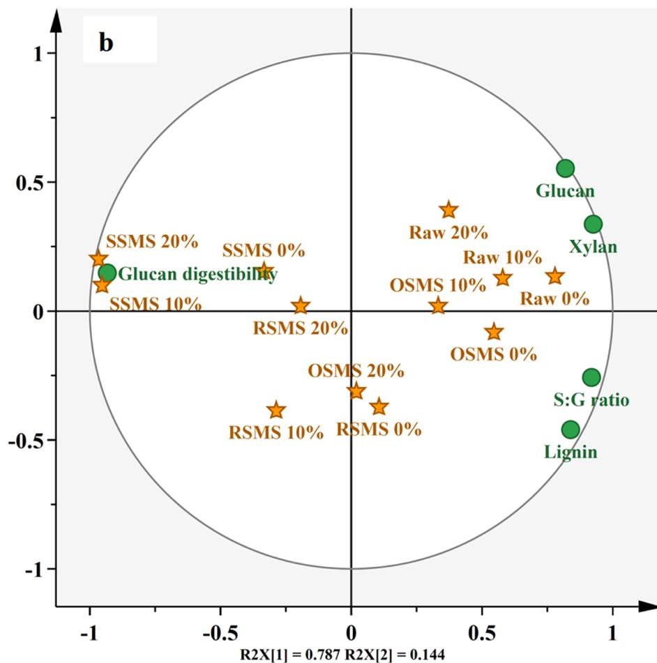
**Fig. 5.** Enzymatic digestibility (a) of glucan contained in the raw substrates and SMSs (mean ± SE). \* indicates significant differences ( $p < 0.05$ ) between treatments. PCA biplot (b) showing the major chemical components of substrates and glucan digestibility. Each star represents an observation. Raw: raw substrate; SSMS: shiitake-based SMS; OSMS: oyster-based SMS; RSMS: reishi-based SMS.
