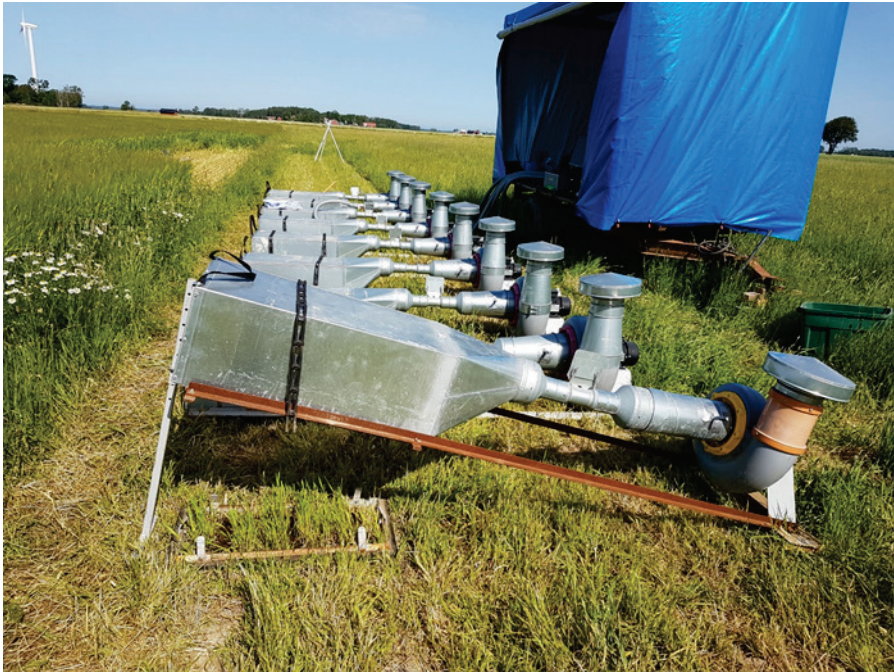
Figure 4. Setup for the ammonia emission experiments. The nine wind tunnels were connected to online ammonia measurements with a cavity ring-down spectrometer.
