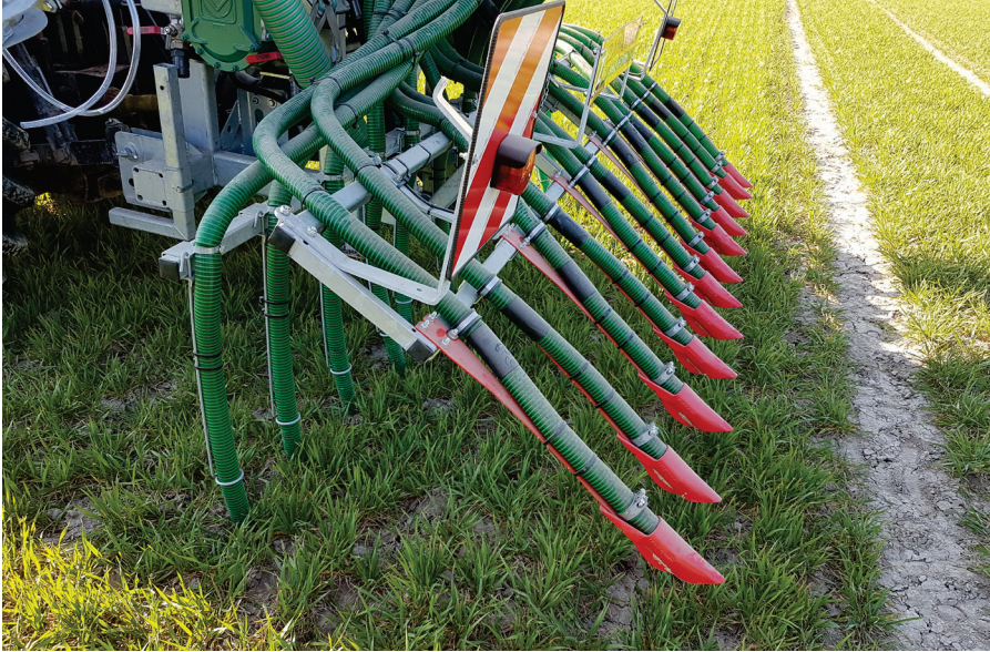
Figure 1. Slurry spreader (Zunhammer) used in the fertilisation field experiments, equipped with trailing hoses (front row) and trailing shoes (back row).
