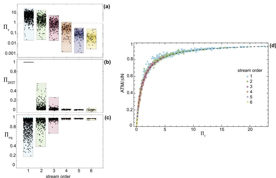
**Figure 2.** Analysis of the IC partitioning for the Susquehanna catchment. (a–c) Governing dimensionless groups for the river reaches (dots) grouped by stream order. (a) Timescale ratio. (b) Relative importance of distributed inputs. (c) Equilibrium ratio. (d) IC partitioning as a function of the timescale ratio. The partitioning is for the fraction of out-of-equilibrium carbon,  $\Delta IN = IN(1 - \Pi_{eq})$ . The dashed line is  $1/(1 + \Pi_\tau^{-1})$ .
