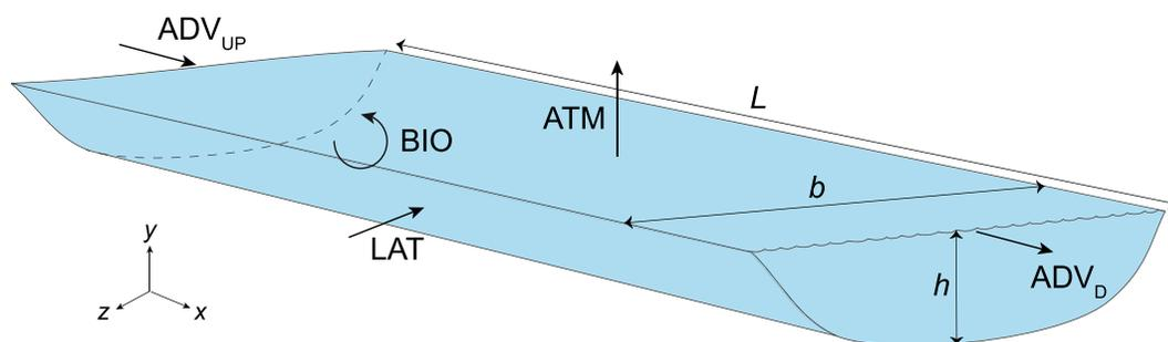
**Figure 1.** Sketch of the inorganic carbon fluxes in a river reach.  $ADV_{UP}$  and  $ADV_D$  are upstream and downstream advection, respectively; ATM is the evasion flux to the atmosphere; BIO is the net difference between organic matter decomposition and net primary production; LAT is the lateral input. In the text, total distributed inputs are defined as  $DIST = LAT + BIO$ .
