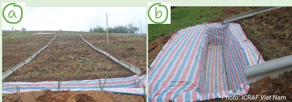
Figure 2. (a) Protective fence made of fiber-cement sheets at measuring areas for soil erosion, (b) The dimensions of the soil trap is 0.5m wide and 0.8m depth below each erosion plot.
