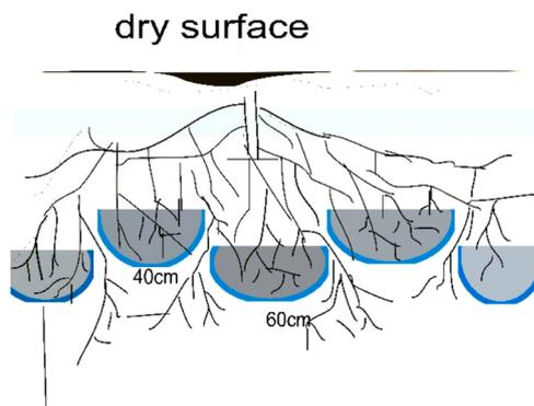
**Fig. 3.** Sub-surface water retention technology (SWRT) system, consisting of U-shaped polyethylene membranes installed at two depths (40 cm and 60 cm) below the root growth zone to create an artificial water table, increasing water and nutrient availability and reducing leaching losses.
