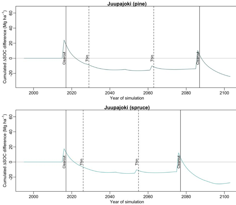
**FIGURE 3** | Comparison of the SOC differences (mean over each MCMC) over time between the two alternative scenarios (cumulated  $\Delta$ SOC of the clear-cut minus cumulated  $\Delta$ SOC of the set-aside scenario). Positive values mean that the clear-cut sequesters more C than the set-aside scenario.
