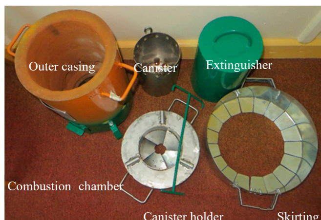
Figure 1. GASTOV gasifier cookstove. Fuel is placed in the canister, which is placed inside the outer casing, with the combustion chamber and skirting on top. The canister holder is used to lift the canister. At the end of cooking, the canister is removed and the extinguisher is placed on top to cut off the oxygen supply.
