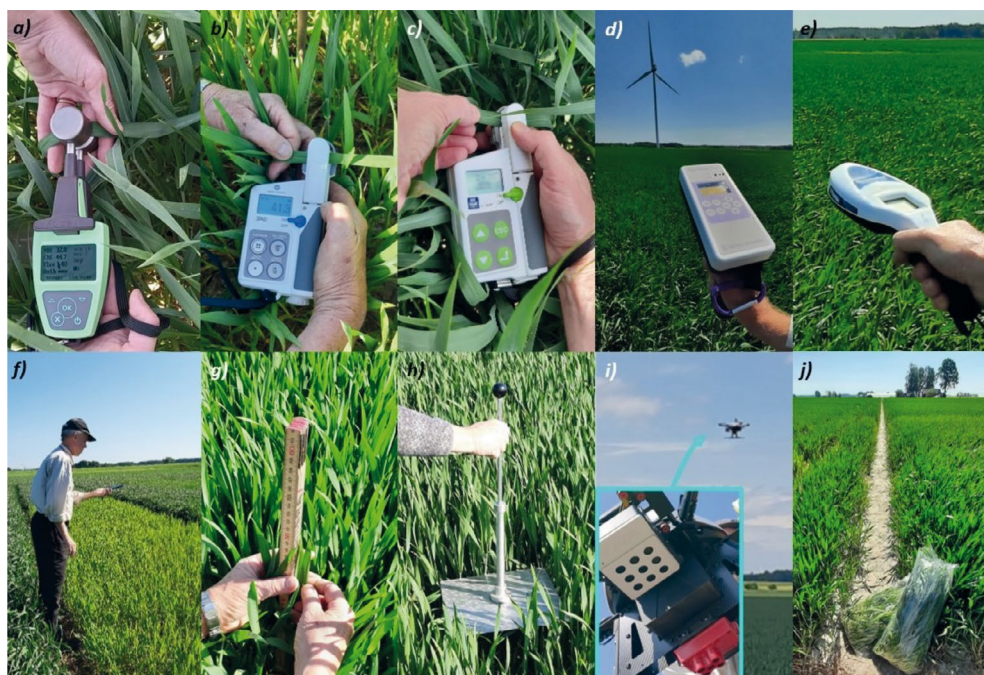
Figure 2. Equipment used in 2024. (a) Dualex, (b) SPAD, (c) N-tester, (d) RapidScan, (e) GreenSeeker, (f) Canopeo, (g) ruler, (h) platometer, (i) drones, two different sensors, and (j) cut crop samples for determination of fresh weight and N uptake.
