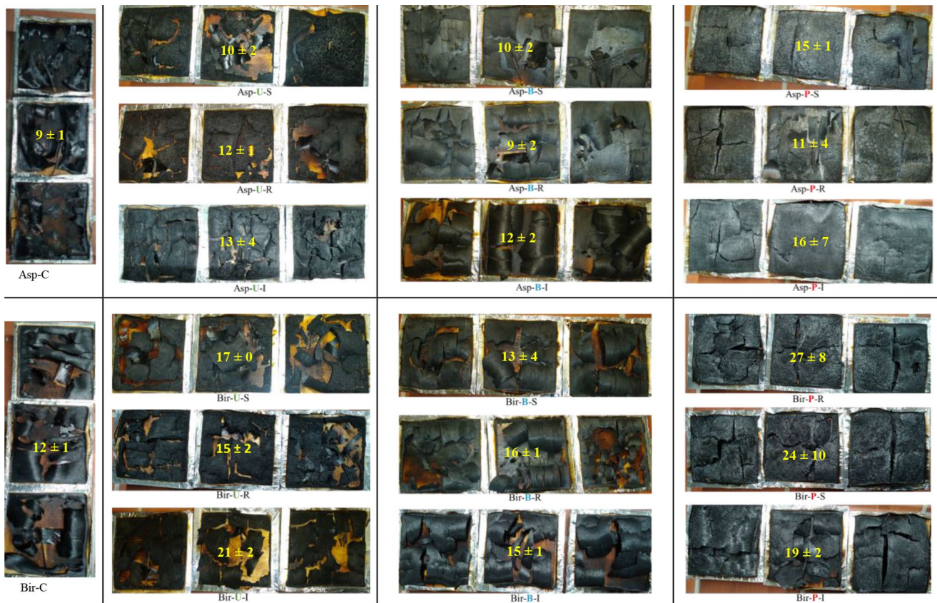
Fig. 6 Veneer residues (values represent TTI) after exposure to 50 kW/m 2 radiant heat from cone heater of a cone calorimeter
