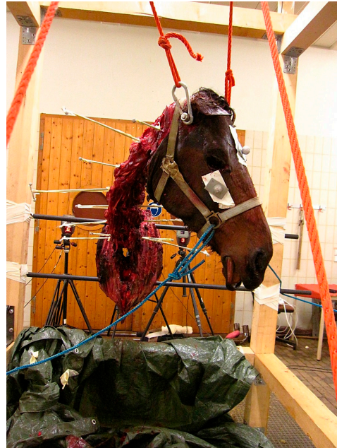
Figure 3. Original lab setting of a head and neck segment during lateral bending to the left, secured in the measurement frame with steel rods between the fifth and sixth rib. Ropes running through a pulley system are attached to a transverse bolt through the base of the skull to suspend the head. T-bar pins are visible in each cervical and the first thoracic vertebra, the side of the T piece and the single points are alternating. On all three end points of the T-bar pins, reflective, spherical kinematic markers are attached. The kinematic markers on the right facial crest and on the frontal bone are visible. Ropes attached to the headcollar were used to achieve head and neck movements. The specimen is of horse L, part of the larger study group.
