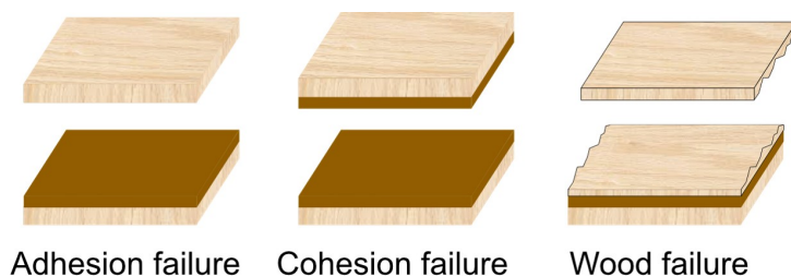
Figure 9. Schematic representation of failure modes.
