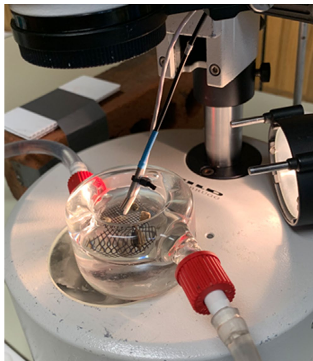
FIGURE 4 Custom-built glass chamber including a shallow well (20 mL volume) to assess CT_{max} of aquatic embryos or larvae. The chamber is a well in an enclosed water bath (heating mantle) heated by water pumped through the red nozzles. Embryos are at the bottom of the well, inside a fine mesh, kept in place by small pebbles. Larvae can be tested in the same arena without a mesh. The heating mantle is placed on a stereomicroscope, attached to a camera, to monitor individual movement. An optical oxygen probe and temperature sensor are placed in the animal arena without blocking the view of the embryos or larvae.
