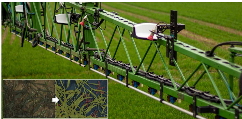
Figure 6 Cameras for weed detection, mounted on a spray boom. Images are taken continuously and analysed for weed and crop coverage in real time. Inset: original image (left) and classified image (right). Source: Photo adapted from: Dimensions Agri Technologies, Norway.
