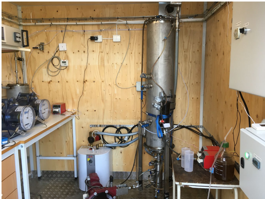
Figure 6. TBR setup A ( V_{pbv} = 35 L) with assembled equipment.
