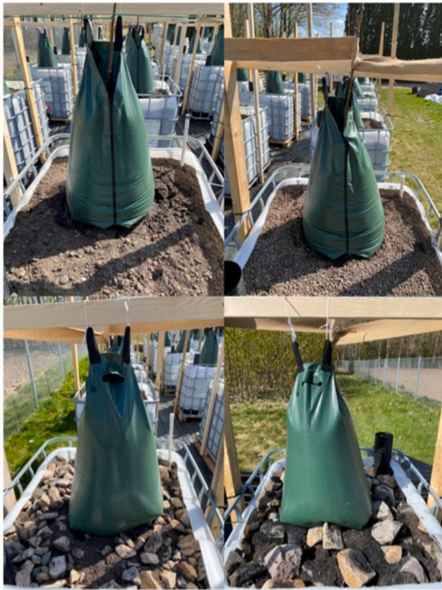
Fig. 1. The four different substrates, immediately after the planting of the trees and the installation of irrigation bags. Upper left is AMA, upper right is PU, lower left is SM and lower right is RM.
