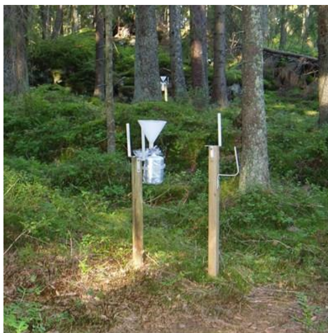
FIGURE 11: AN EXAMPLE OF A SUITABLE COLLECTOR FOR SAMPLING DEPOSITION
