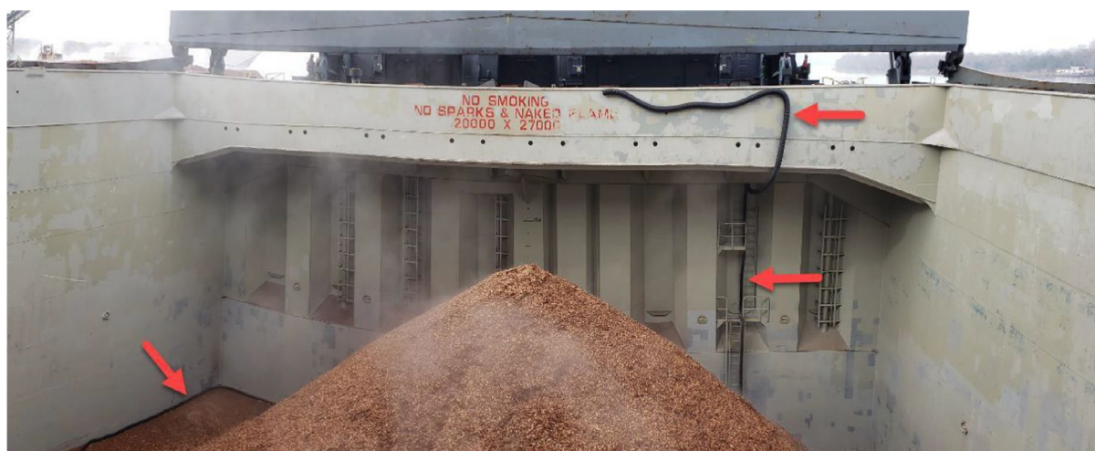
FIGURE 2 Shiphold with recirculation tubing (indicated by red arrows).
