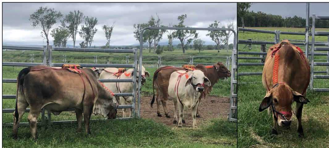
Fig. 1. Heifers wearing the saddle and halter equipment designed to link the sampling canister to the animals' noses to collect a sample of respired gas. Note that the coiled tubing is the key under pasture conditions to permit a full range of movement for the grazing animal.
