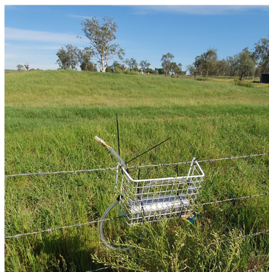
Fig. 2. Environmental canister with tubing and inlet attached to paddock fence at the University of Queensland Gatton campus, Gatton, Queensland. This picture also showcases the pasture where the animals were kept.
