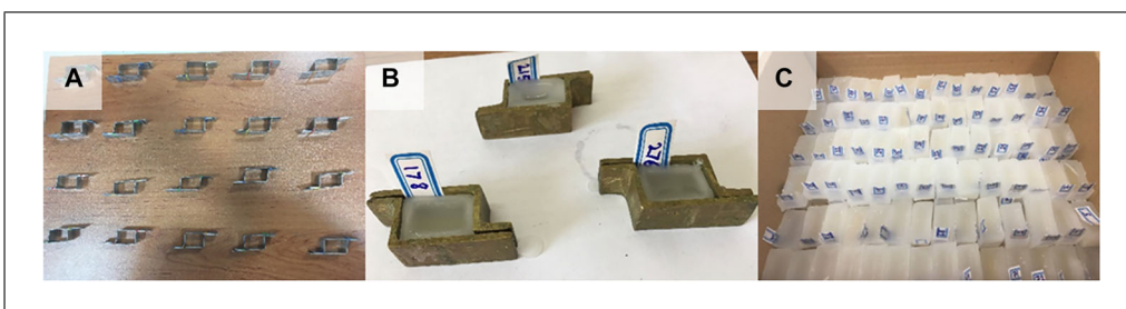
Figure 2 Molds and paraffin blocks. (A) Paraffin molds made of brass; each assembled mold contains two pieces of surface-smoothened, bent metal in the shape of the Latin letter L. (B) Labeled paraffin molds containing the desired sample. (C) Paraffin blocks containing different stem specimens that have been removed from the molds.
