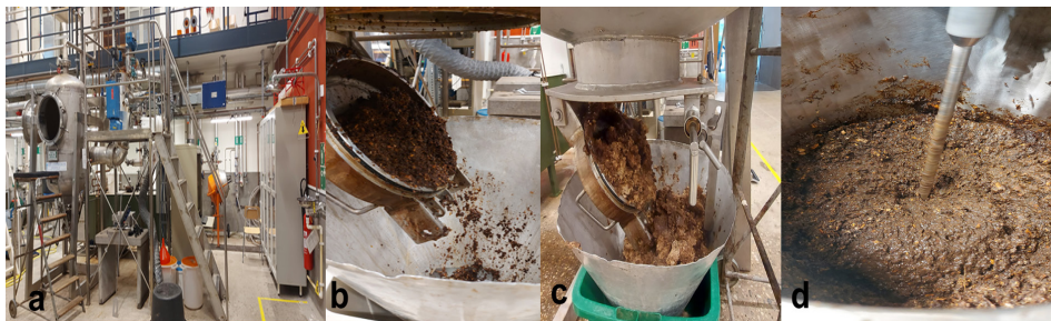
Figure 7. Conversion of cassava residues in hydrolysates (Adapted from Paper II ). (a) Pretreatment unit for steam expansion (STEX) of the lignocellulosic biomass at Lund University, Sweden; (b-c) Biomass after STEX; (d) Enzymatic hydrolysis applied for cassava biomass.
