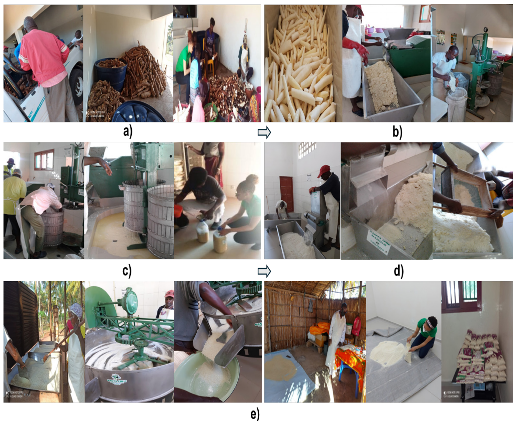
Figure 4. Main steps in cassava roasted flour ( rale ) processing at small-scale units in Inhambane: (a) root reception and peeling; (b) grating and pressing, (c) fermentation and liquid drainage; (d) sieving and drying; (e) roasting, packaging, and storage of final product (Adapted from Paper I ).
