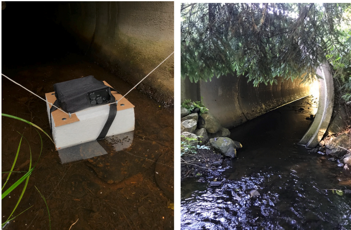
Fig. 2. The ultrasound detector (Pettersson D500X) was placed on a small raft (left) and placed within the pipe culvert (right). There was no directional horn on the detector and consequently also bats foraging behind and above the detector was recorded. Photo: Johnny de Jong.
