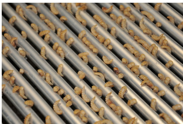
FIGURE 4 A bar sieve or fish grader, used to sieve pupae from the larvae.
