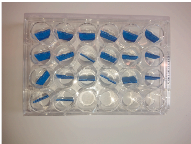
Fig. 1. Autoclaved coupons (1 × 1.5 cm) of conveyor belt material placed vertically in a 24-well plate prior to the addition of bacterial suspensions.
