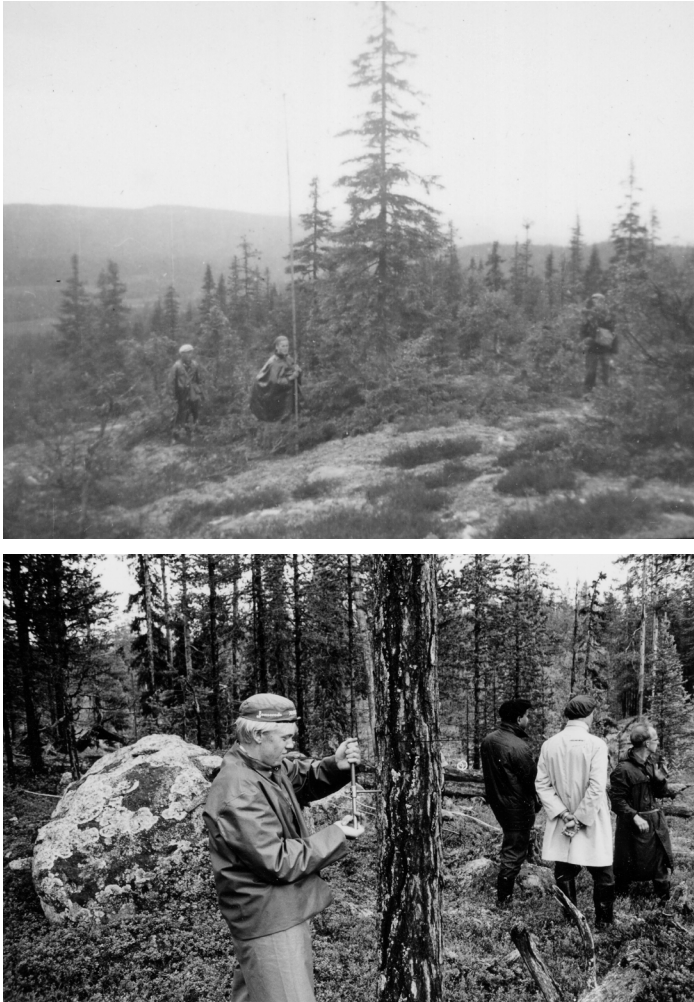
Figure 2. Top: Swedish National Forest Inventory (NFI) fieldwork in Jämtland, c. 1939; Bottom: Collecting tree cores in Norrbotten, c. 1966. Source: SLU Media Bank.
