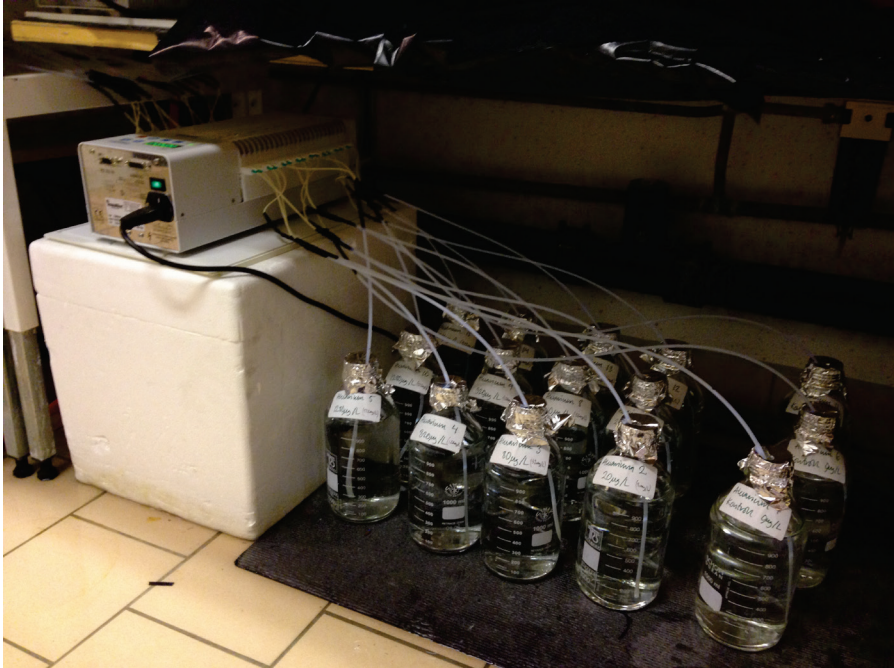
Figure 3. Exposure bottles delivering NSAID via a peristaltic pump.
