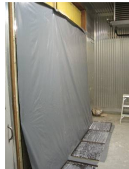
Figure 23. Plastic film was draped over the wall on both sides, leaving an air cavity between wall and plastic. This prevented the wall from drying too quickly.
