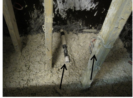
Figure 19. Probe for RH and temperature sensor (left arrow) and electrodes inside the wooden studs (right arrow).
