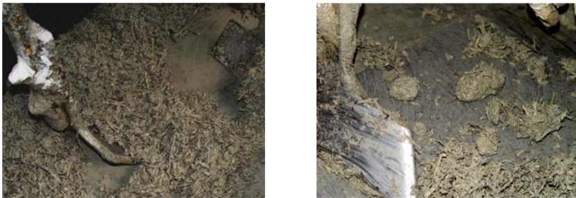
Figure 15. Mixing of LHC. On the left LHC with only shiv, on the right LHC with both shiv and fibres. Balling of the material is clearly visible in the right-hand diagram. (Picture: Nguyen, (2009))
