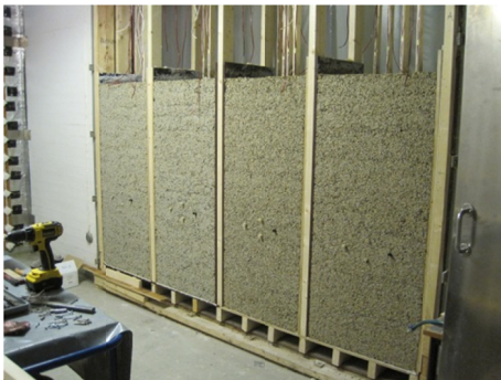
Figure 22. The wall after the shuttering plywood had been removed. Probes for RH and temperature sensors in the centre of the walls.
