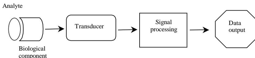
Figure 1. Schematic illustration of the components of a biosensor.
