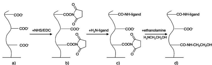
Figure 5. Amine coupling of ligand to a sensor surface: a) Non-activated carboxyl groups on the dextran; b) The carboxyl groups are activated by addition of a mixture of succinimide (NHS) and carbodiimide (EDC); c) The ligand is covalently bound to the sensor surface; d) Remaining esters are deactivated by addition of ethanolamine (Johnsson, Löfås & Lindquist, 1991).
