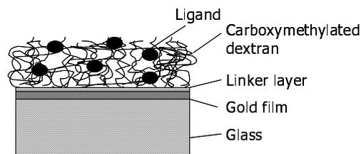
Figure 4. A schematic figure of a Biacore sensor surface in cross-section. The surface consists of a piece of glass covered with a thin gold film. Onto the metal film a linker layer is attached to which a coupling matrix, such as the carboxymethylated dextran layer, is bound.
