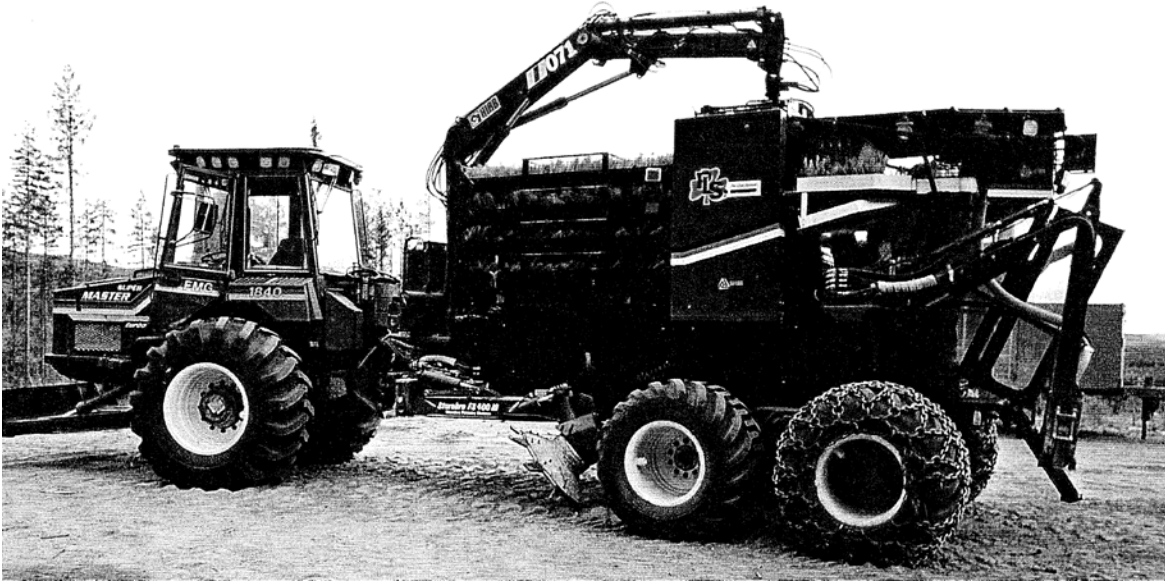
Figure 20. The final version of the Silva Nova planting machine (from Åhlund 1995).
