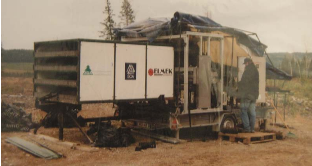
Figure 29. The portable loading robot at a roadside landing in 1998. The nursery trays were fed in by a conveyor belt (at right of the operator), and the loaded PLS belts were automatically arranged into separate slots within the white coloured container at left (from Lantz, Pers. Comm.).
