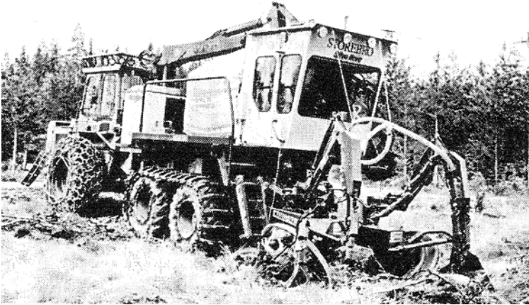
Figure 16. The MoDo Mekan planting machine (from Malmberg 1990).
