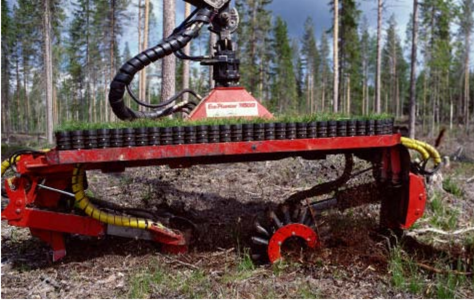
Figure 24. The EcoPlanter planting head (from Normark & Norr 2002)
