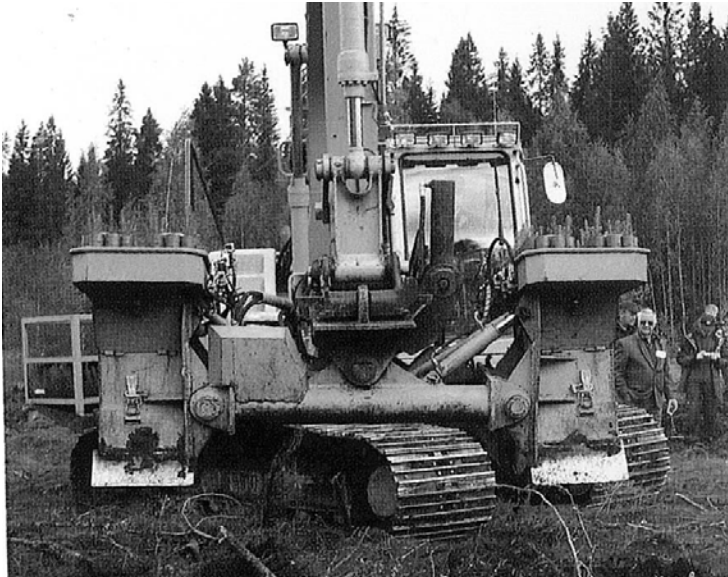
Figure 26. The M-Planter mounted on an excavator (from Johansson 2007)
