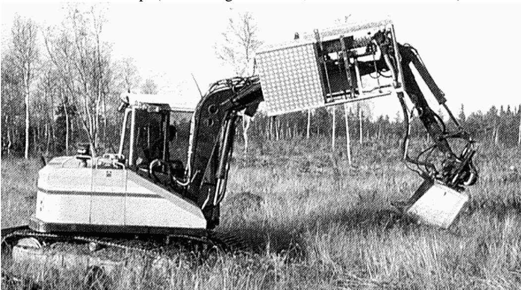
Figure 25. The SwePlant prototype mounted on a medium-sized excavator (from Hallonborg et al. 1997)
