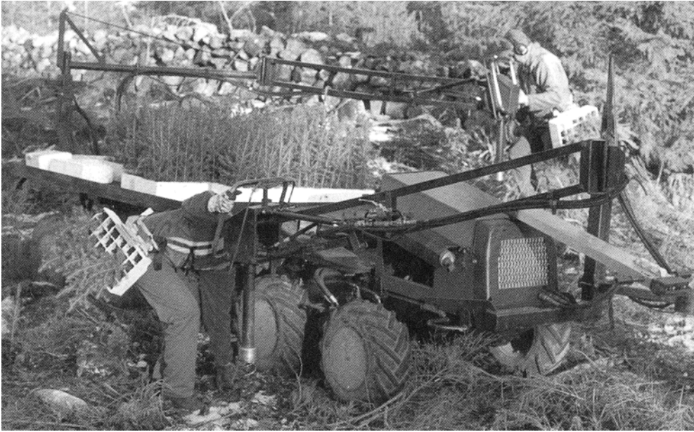
Figure 27. The Hevotrac partially mechanized planting machine (from Hallonborg et al. 1997)
