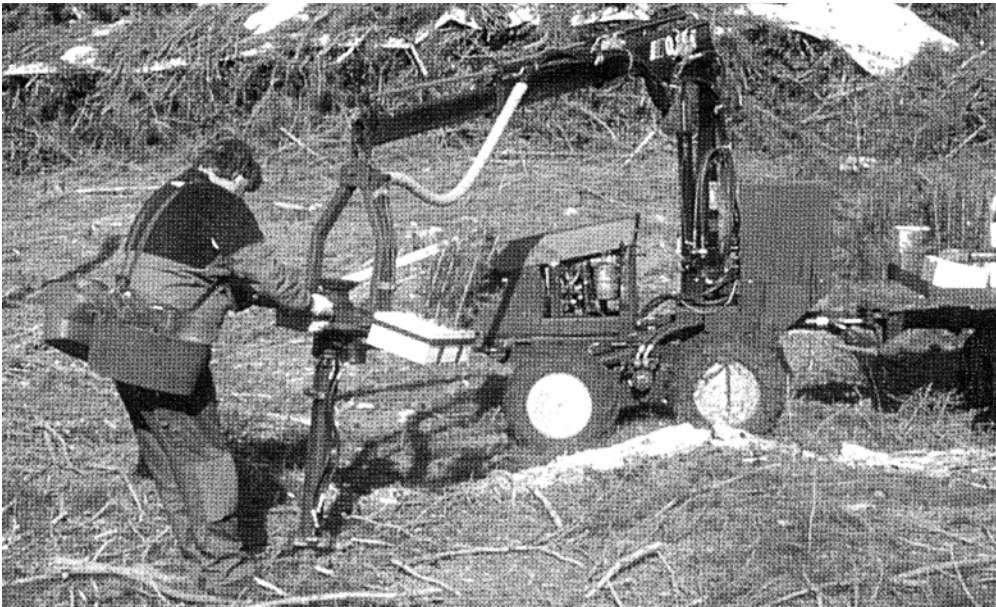
Figure 28. The Silviplant partially mechanized planting machine (from Hallonborg et al. 1997)
