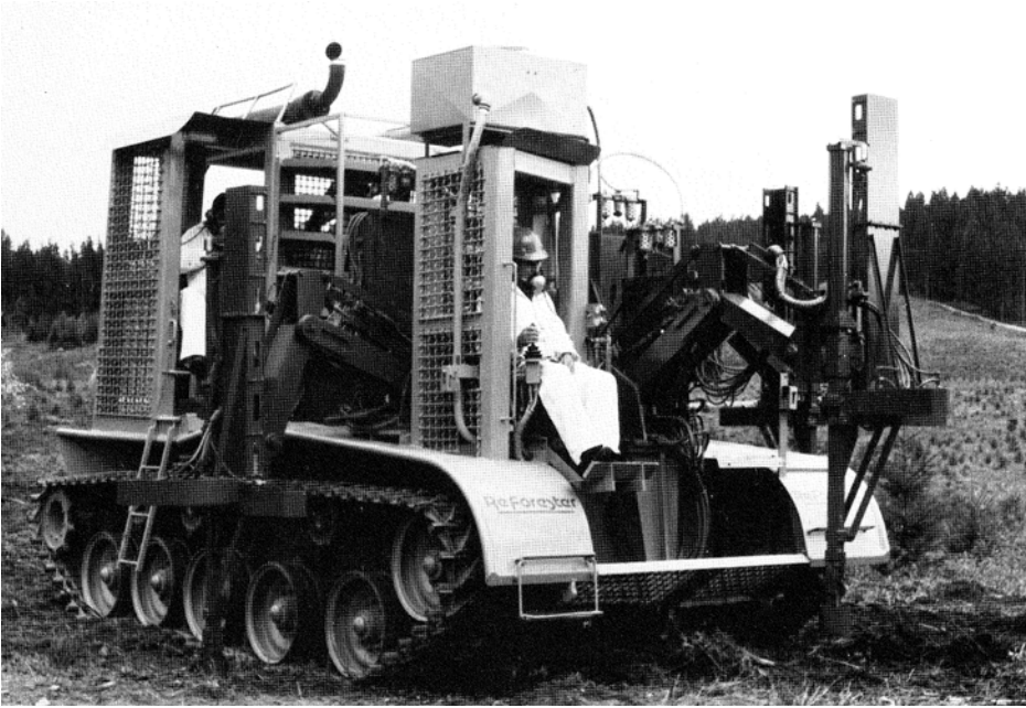
Figure 19. The ReForester prototype automatic injection planting machine (from Walters & Silversides 1979).
