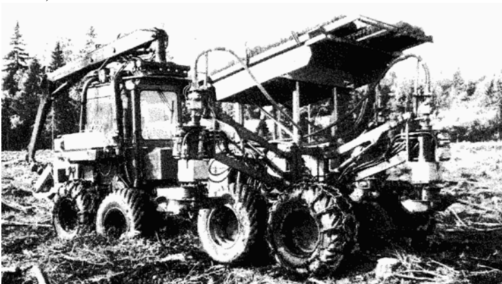
Figure 21. The HIKO intermittently advancing planting machine (from Berg 1983).
