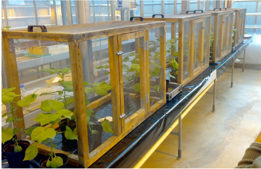
Figure 3. Laboratory setup to test the influence of HIPVs on the oviposition behaviour in S. littoralis (Zakir et al., 2012).
