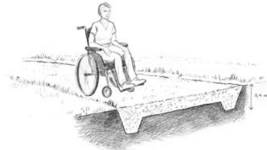
Fig 6.1:1 Path with runoff drains
