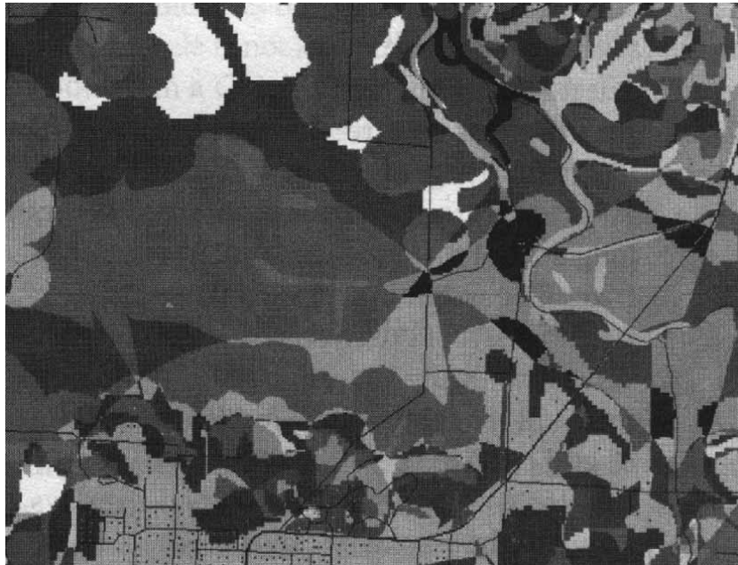
Figure 10. Standard suitability map, using the McHarg method. Many colors and slivers make it hard to read. (Hanna and Culpepper, 1998)
